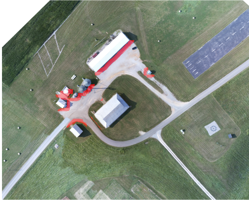
Figure 3.10: Region of interest overlay, showing intersections between buildings and roads highlighted in red on a map to help the user choose POI for investigation.
