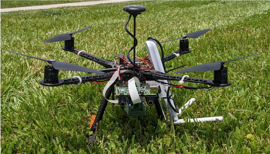
Figure 3.3: Holybro S-500 drone with payload. The LAI is shown, but HAS is nearly identical.
