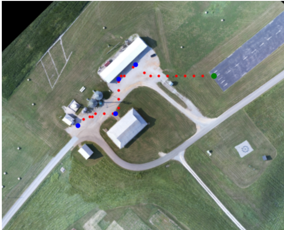
(c) Drone (green dot) path, where red dots are the waypoints and blue dots are POI.
