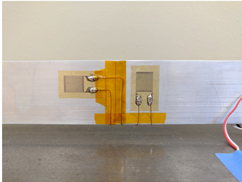
Figure 4.10: Photo of the strain gages used to measure the ground-truth stress in the beam.
