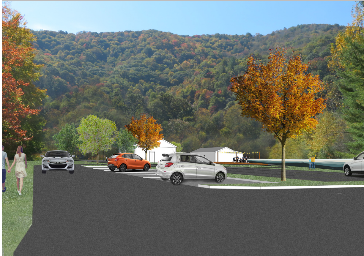
Perspective 2: Parking Lot with Permeable Paving. The new parking lot can utilize permeable paving within the parking stalls to reduce stormwater run off and minimize the migration of pollutants into the nearby creek. The redeveloped visitors center and outdoor performance area can be seen in the background.
