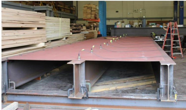
Figure 7-1. Accelerometers at midspan
