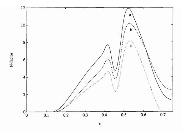
Figure 23. Variation of the N-factor for the most dangerous frequency with streamwise position for hump # 3 located at L3 and all three Mach numbers: a)  $F=35x10^{-6}$  when M=0.14, b)  $F=30x10^{-6}$  when M=0.50, and c)  $F=30x10^{-6}$  when M=0.65;  $h_3=8.0\times10^{-4}$  and L3 ( $x_\ell=0.40$  and  $x_r=0.50$ ).
