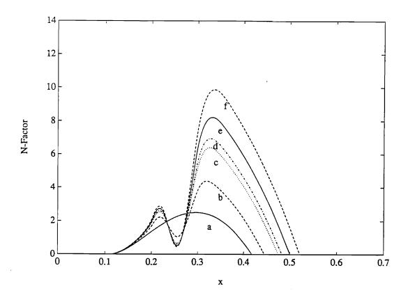
Figure 19. Variation of the N-factor for the most dangerous frequency with streamwise position when M=0.65 for six heights at location L1: a)  $h_0$  clean airfoil, b)  $h_1=5.0\times 10^{-4}$ , c)  $h_2=7.5\times 10^{-4}$ , d)  $h_3=8.0\times 10^{-4}$ , e)  $h_4=9.0\times 10^{-4}$ , and f)  $h_5=1.0\times 10^{-3}$ ;  $F=40\times 10^{-6}$  and L1 ( $\chi_\ell=0.20$  and  $\chi_r=0.30$ ).
