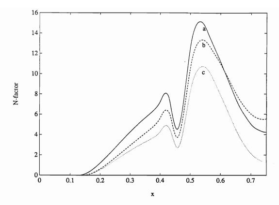
Figure 25. Variation of the N-factor for the most dangerous frequency with streamwise position for hump # 5 located at L3 and all three Mach numbers: a)  $F=35x10^{-6}$  when M=0.14, b)  $F=30x10^{-6}$  when M=0.50, and c)  $F=30x10^{-6}$  when M=0.65;  $h_5=1.0\times10^{-3}$  and L3 ( $x_\ell=0.30$  and  $x_r=0.40$ ).
