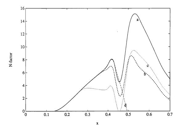
Figure 27. Variation of the N-factor for the most dangerous frequency with streamwise position for three suction location when M = 0.14 a) no suction, b)  $S_1: x=0.34$  to 0.54, c)  $S_2: x=0.27$  to 0.44, and d)  $S_3: x=0.42$  to 0.59;  $F=35\times 10^{-6}$ ,  $C_q=1.5\times 10^{-4}$ ,  $h_5=1.0\times 10^{-3}$ , and L3 ( $x_\ell=0.40$  and  $x_r=0.50$ ).
