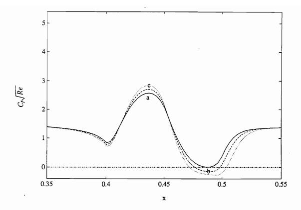
Figure 12. Variation of the skin-friction coefficient with streamwise position for humps # 3,4,5 located at L3 when M = 0.50: a)  $h_3 = 8.0 \times 10^{-4}$ , b)  $h_4 = 9.0 \times 10^{-4}$ , and c)  $h_5 = 1.0 \times 10^{-3}$ ; L3 ( $x_{\ell} = 0.40$  and  $x_{\ell} = 0.50$ ).
