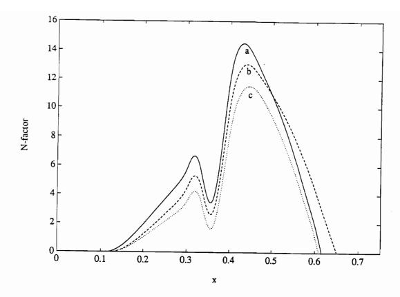
Figure 22. Variation of the N-factor for the most dangerous frequency with streamwise position for hump # 5 located at L2 and all three Mach numbers: a)  $F = 40 \times 10^{-6}$  when M = 0.14, b)  $F = 40 \times 10^{-6}$  when M = 0.50, and c)  $F = 35 \times 10^{-6}$  when M = 0.65;  $h_5 = 1.0 \times 10^{-3}$  and L2 ( $x_{\ell} = 0.30$  and  $x_r = 0.4$ ).
