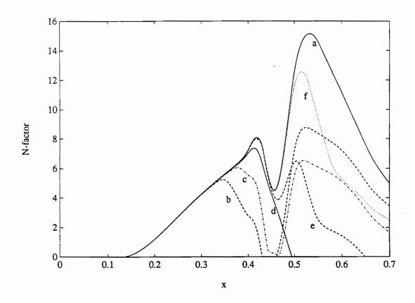
Figure 29. Variation of the N-factor for the most dangerous frequency with streamwise position for different locations of a suction strip of width 0.08: a) no suction, b)  $S_1: x = 0.34$  to 0.42, c)  $S_2: x = 0.37$  to 0.45, d)  $S_3: x = 0.40$  to 0.48, e)  $S_4: x = 0.45$  to 0.53, and f)  $S_5: x = 0.49$  to 0.57;  $F = 35 \times 10^{-6}$ ,  $C_q = 4.5 \times 10^{-4}$ , M = 0.14, and L3 ( $x_\ell = 0.40$  and  $x_r = 0.50$ )..
