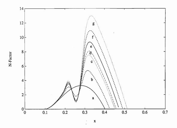
Figure 18. Variation of the N-factor for the most dangerous frequency with streamwise position when M=0.50 for seven heights at location L1: a)  $h_0$  clean airfoil, b)  $h_1 = 5.0 \times 10^{-4}$ , c)  $h_2 = 7.5 \times 10^{-4}$ , d)  $h_3 = 8.0 \times 10^{-4}$ , e)  $h_4 = 9.0 \times 10^{-4}$ , f)  $h_5 = 1.0 \times 10^{-3}$ , g)  $h_6 = 1.2 \times 10^{-3}$ ; and  $F = 45 \times 10^{-6}$  and L1 ( $x_\ell = 0.20$  and  $x_r = 0.30$ ).
