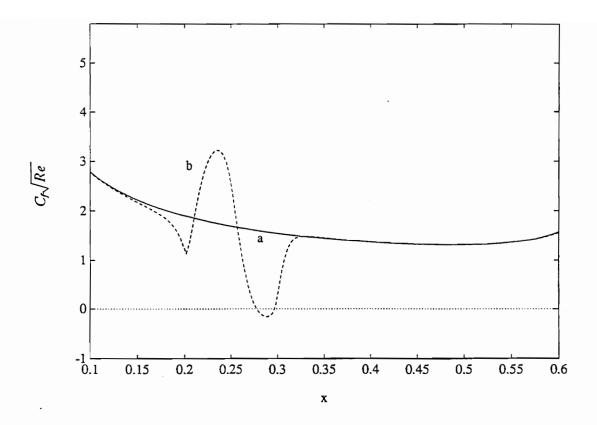
Figure 13. Variation of the skin-friction coefficient with streamwise position for the clean airfoil and hump # 5 located at L1: a) clean airfoil, b)  $h_3 = 1.0 \times 10^{-3}$ ; M = 0.50 and L1 (  $x_{\ell} = 0.20$  and  $x_{r} = 0.30$ ).
