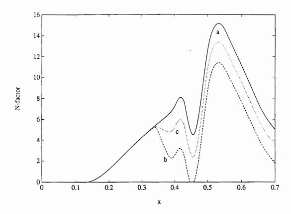
Figure 33. Variation of the N-factor for the most dangerous frequency with streamwise position for three cooling levels when M = 0.14: a) no cooling, b)  $T_w/T_{ad}=0.8$ , and c)  $T_w/T_{ad}=0.9$ ;  $F=35\times 10^{-6}$ , cooling extends from x=0.34 to 0.38,  $h_5=1.0\times 10^{-3}$ , and L3 ( $x_\ell=0.40$  and  $x_r=0.50$ ).
