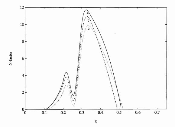
Figure 16. Variation of the N-factor for the most dangerous frequency with streamwise position for hump # 5 located at L1 and all three Mach numbers: a)  $F = 45 \times 10^{-6}$  when M = 0.14, b)  $F = 45 \times 10^{-6}$  when M = 0.50, and c)  $F = 40 \times 10^{-6}$  when M = 0.65;  $h_5 = 1.0 \times 10^{-3}$  and L1 ( $x_\ell = 0.20$  and  $x_r = 0.30$ ).
