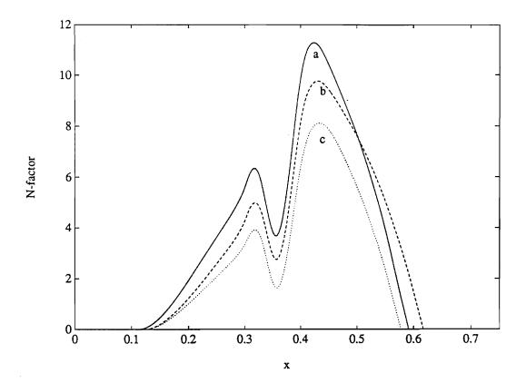
Figure 20. Variation of the N-factor for the most dangerous frequency with streamwise position for hump # 3 located at L2 and all three Mach numbers: a)  $F = 40 \times 10^{-6}$  when M = 0.14, b)  $F = 40 \times 10^{-6}$  when M = 0.50, and c)  $F = 35 \times 10^{-6}$  when M = 0.65;  $h_3 = 8.0 \times 10^{-4}$  and L2 ( $x_\ell = 0.30$  and  $x_r = 0.40$ ).
