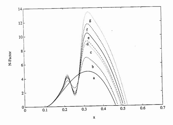
Figure 17. Variation of the N-factor for the most dangerous frequency with streamwise position when M=0.14 for seven heights at location L1: a)  $h_0$  clean airfoil, b)  $h_1 = 5.0 \times 10^{-4}$ , c)  $h_2 = 7.5 \times 10^{-4}$ , d)  $h_3 = 8.0 \times 10^{-4}$ , e)  $h_4 = 9.0 \times 10^{-4}$ , f)  $h_5 = 1.0 \times 10^{-3}$ , and g)  $h_6 = 1.2 \times 10^{-3}$ ;  $F = 45 \times 10^{-6}$  and L1 ( $x_c = 0.20$  and  $x_r = 0.30$ ).
