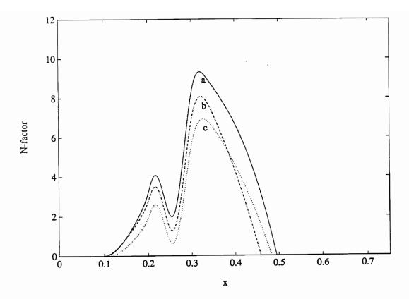
Figure 14. Variation of the N-factor for the most dangerous frequency with streamwise position for hump # 3 located at L1 and all three Mach numbers: a)  $F = 45 \times 10^{-6}$  when M = 0.14, b)  $F = 45 \times 10^{-6}$  when M = 0.50, and c)  $F = 40 \times 10^{-6}$  when M = 0.65;  $h_3 = 8.0 \times 10^{-4}$  and L1 ( $x_\ell = 0.2$  and  $x_r = 0.3$ ).
