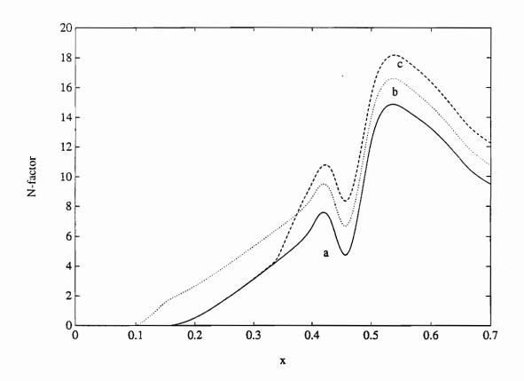
Figure 35. Variation of the N-factor for the most dangerous frequency with streamwise position for hump # 5 located at L3 and two heating strips: a) no heating, b) x = 0.09 to 0.140, and c) x = 0.34 to 0.38;  $F = 30 \times 10^{-6}$ ,  $T_w/T_{ad} = 1.3$ ,  $h_5 = 1.0 \times 10^{-3}$ , M = 0.14, and L3 ( $x_{\ell} = 0.40$  and  $x_r = 0.50$ ).
