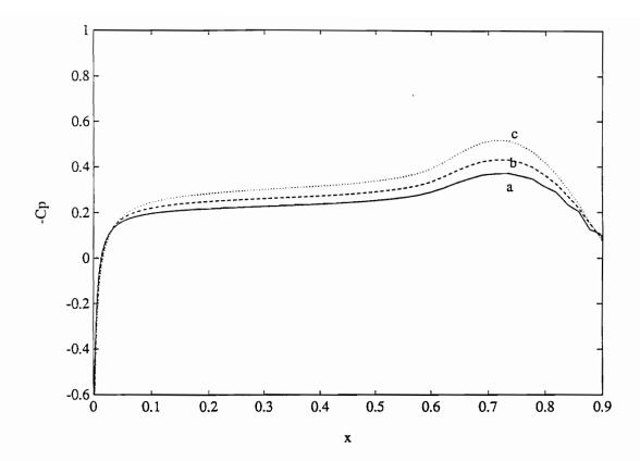
Figure 2. Pressure distributions for the EQH1260 airfoil calculated by using an Euler code: a) M=0.14, b) M=0.50, and c) M=0.65.
