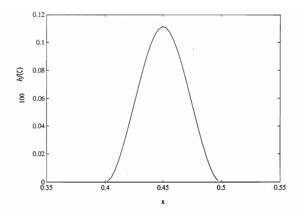
Figure 3. Shape of the considered cubic hump located at L3:  $h_5=1.0\times 10^{-3}$  and L3 (  $x_\ell=0.40$  and  $x_r=0.50$ ).
