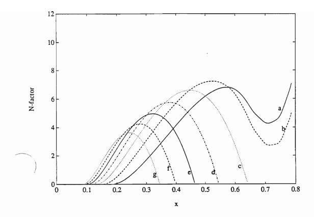
Figure 4. Variation of the N-factor with streamwise position for the clean airfoil when M = 0.14 for several frequencies: a)  $F = 25 \times 10^{-6}$ , b)  $F = 30 \times 10^{-6}$ , c)  $F = 35 \times 10^{-6}$ , d)  $F = 40 \times 10^{-6}$ , e)  $F = 45 \times 10^{-6}$ , f)  $F = 50 \times 10^{-6}$ , and g)  $F = 55 \times 10^{-6}$ .
