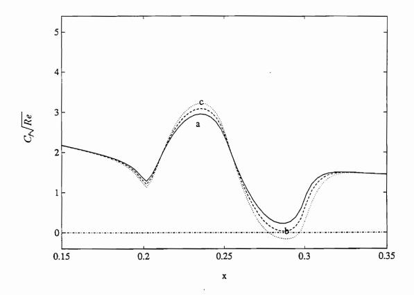
Figure 9. Variation of the skin-friction coefficient with streamwise position for humps # 3,4,5 located at L1 when M = 0.50: a)  $h_3 = 8.0 \times 10^{-4}$ , b)  $h_4 = 9.0 \times 10^{-4}$ , and c)  $h_5 = 1.0 \times 10^{-3}$ ; L1 ( $x_{\ell} = 0.20$  and  $x_{r} = 0.30$ ).
