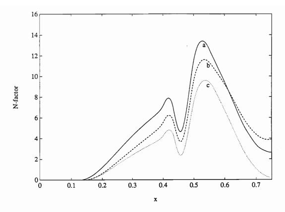
Figure 24. Variation of the N-factor for the most dangerous frequency with streamwise position for hump # 4 located at L3 and all three Mach numbers: a)  $F=35x10^{-6}$  when M=0.14, b)  $F=30x10^{-6}$  when M=0.50, and c)  $F=30x10^{-6}$  when M=0.65;  $h_4=9.0\times10^{-4}$  and L3 ( $x_\ell=0.30$  and  $x_r=0.40$ ).
