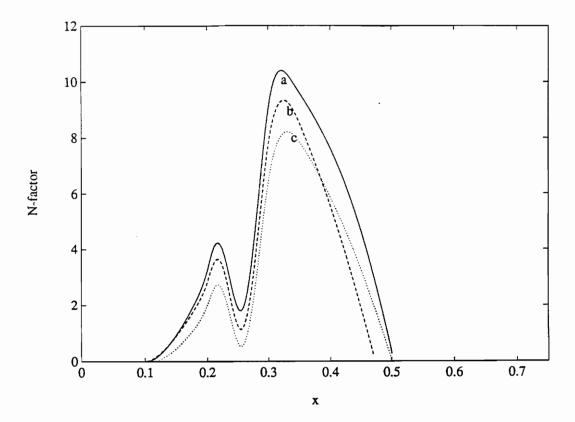
Figure 15. Variation of the N-factor for the most dangerous frequency with streamwise position for hump # 4 located at L1 and all three Mach numbers: a)  $F=45\times10^{-6}$  when M=0.14, b)  $F=45\times10^{-6}$  when M=0.50, and c)  $F=40\times10^{-6}$  when M=0.65;  $h_4=9.0\times10^{-4}$  and L1 ( $x_\ell=0.20$  and  $x_r=0.30$ ).
