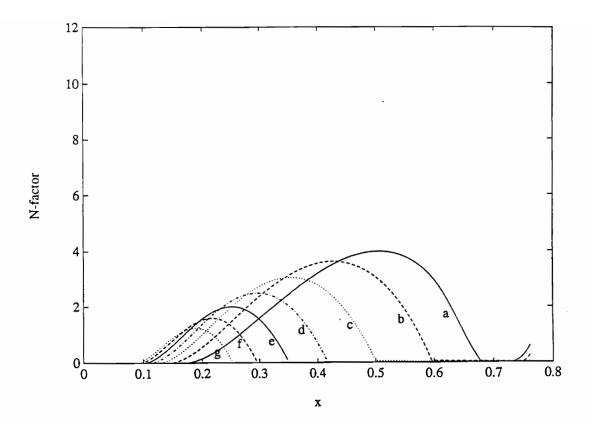
Figure 6. Variation of the N-factor with streamwise position for the clean airfoil when M = 0.65 for several frequencies: a)  $F = 25 \times 10^{-6}$ , b)  $F = 30 \times 10^{-6}$ , c)  $F = 35 \times 10^{-6}$ , d)  $F = 40 \times 10^{-6}$ , e)  $F = 45 \times 10^{-6}$ , f)  $F = 50 \times 10^{-8}$ , and g)  $F = 55 \times 10^{-6}$ .
