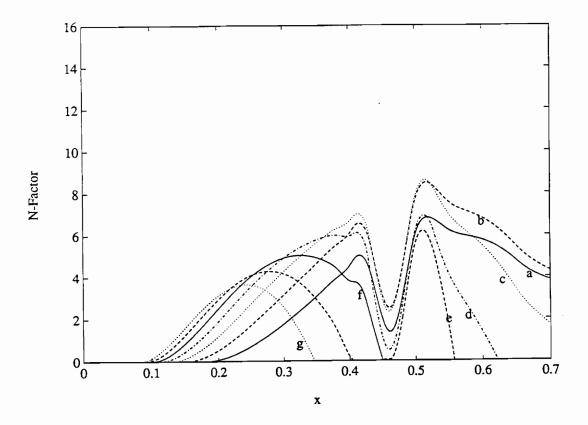
Figure 26. Variation of the N-factor with streamwise position for several frequencies with suction for hump # 5 located at L3 when M = 0.14: a)  $F = 25 \times 10^{-6}$ , b)  $F = 30 \times 10^{-6}$ , c)  $F = 35 \times 10^{-6}$ , d)  $F = 40 \times 10^{-6}$ , e)  $F = 45 \times 10^{-6}$ , f)  $F = 50 \times 10^{-6}$ , and g)  $F = 55 \times 10^{-6}$ ;  $\Delta x_{suction} = 0.37$  to 0.54,  $C_q = 1.5 \times 10^{-4}$ ,  $h_5 = 1.0 \times 10^{-3}$ , and L3 ( $x_\ell = 0.40$  to  $x_r = 0.50$ ).
