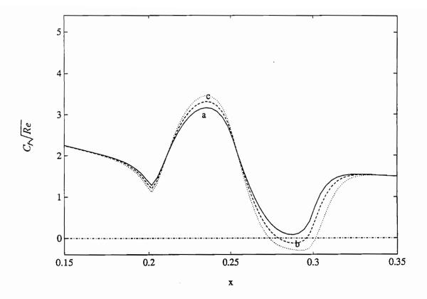
Figure 10. Variation of the skin-friction coefficient with streamwise position for humps # 3,4,5 located at L1 when M = 0.65: a)  $h_3 = 8.0 \times 10^{-4}$ , b)  $h_4 = 9.0 \times 10^{-4}$ , and c)  $h_5 = 1.0 \times 10^{-3}$ ; L1 ( $x_\ell = 0.20$  and  $x_r = 0.30$ ).
