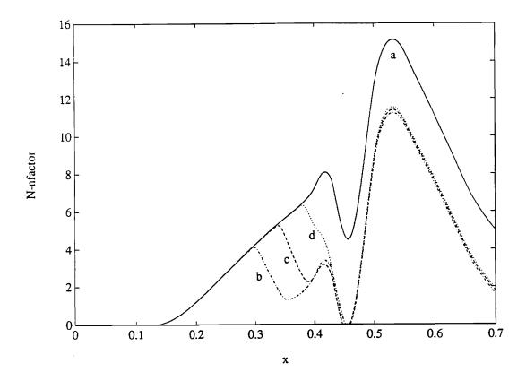
Figure 32. Variation of the N-factor for the most dangerous frequency with streamwise position for three cooling-strip locations when M=0.14: a) no cooling, b)  $C_1: x=0.30$  and 0.34, c)  $C_2: x=0.34$  to 0.38, and d)  $C_3: x=0.38$  to 0.42;  $F=35\times 10^{-6}$ ,  $T_w/T_{ad}=0.8$ ,  $h_5=1.0\times 10^{-3}$ , and L3 ( $x_\ell=0.40$  and  $x_r=0.50$ ).
