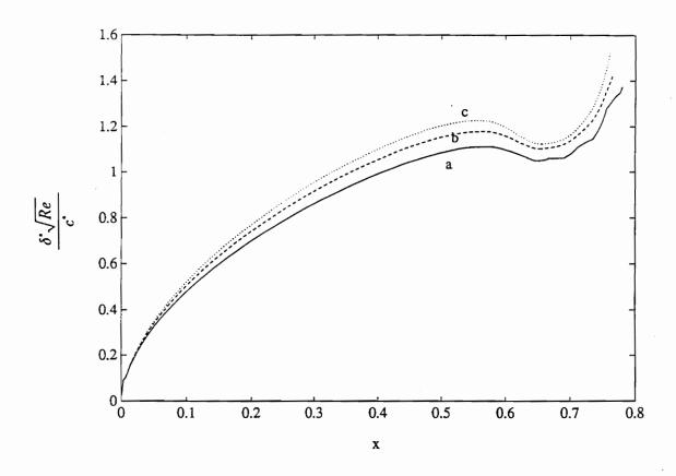
Figure 7. Variation of the displacement thickness with streamwise position for the clean airfoil at three Mach numbers: a) M=0.14, b) M=0.50, and c) M=0.65.
