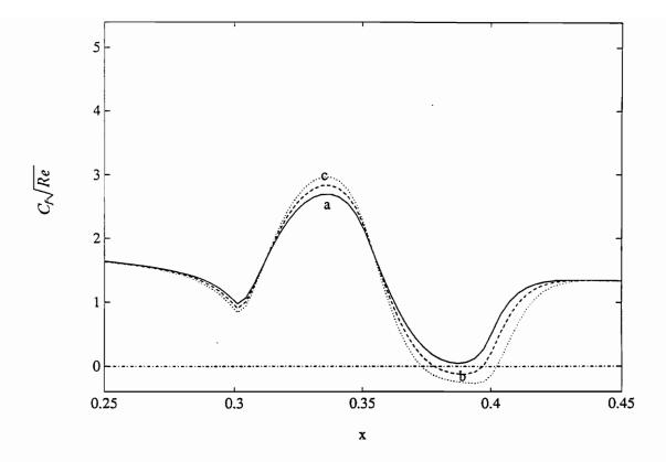
Figure 11. Variation of the skin-friction coefficient with streamwise position for humps # 3,4,5 located at L2 when M = 0.50: a)  $h_3 = 8.0 \times 10^{-4}$ , b)  $h_4 = 9.0 \times 10^{-4}$ , and c)  $h_5 = 1.0 \times 10^{-3}$ ; L2 ( $x_\ell = 0.3$  and  $x_r = 0.4$ ).
