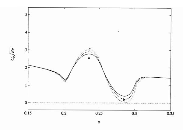
Figure 8. Variation of the skin-friction coefficient with streamwise position for humps # 3,4,5 located at L1 when M = 0.14: a)  $h_3 = 8.0 \times 10^{-4}$ , b)  $h_4 = 9.0 \times 10^{-4}$ , and c)  $h_5 = 1.0 \times 10^{-3}$ ; L1 ( $x_{\ell} = 0.20$  and  $x_{\ell} = 0.30$ ).
