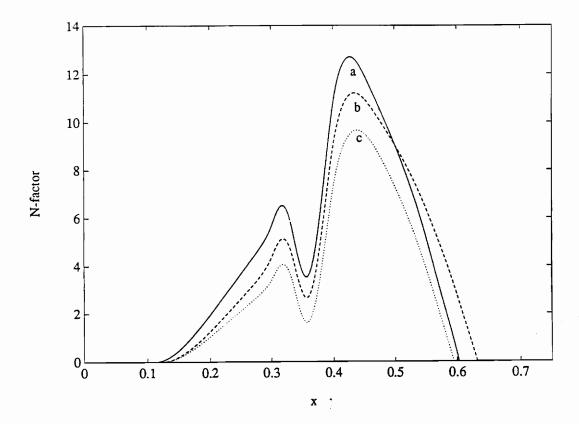
Figure 21. Variation of the N-factor for the most dangerous frequency with streamwise position for hump # 4 located at L2 and all three Mach numbers: a)  $F = 40 \times 10^{-6}$  when M = 0.14, b)  $F = 40 \times 10^{-6}$  when M = 0.50, and c)  $F = 35 \times 10^{-6}$  when M = 0.65;  $h_4 = 9.0 \times 10^{-4}$  and L2 ( $x_\ell = 0.30$  and  $x_r = 0.40$ ).
