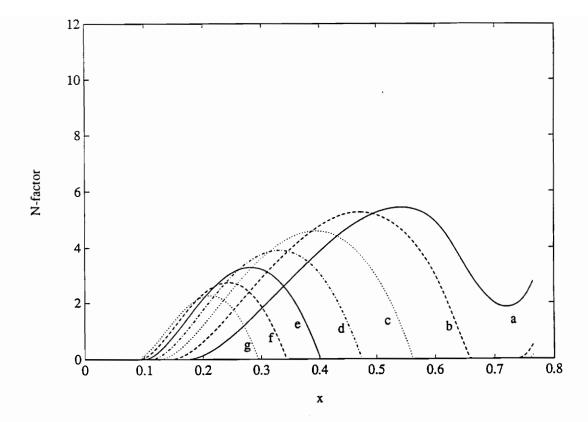
Figure 5. Variation of the N-factor with streamwise position for the clean airfoil when M = 0.50 for several frequencies: a)  $F = 25 \times 10^{-6}$ , b)  $F = 30 \times 10^{-6}$ , c)  $F = 35 \times 10^{-6}$ , d)  $F = 40 \times 10^{-6}$ , e)  $F = 45 \times 10^{-6}$ , f)  $F = 50 \times 10^{-6}$ , and g)  $F = 55 \times 10^{-6}$ .
