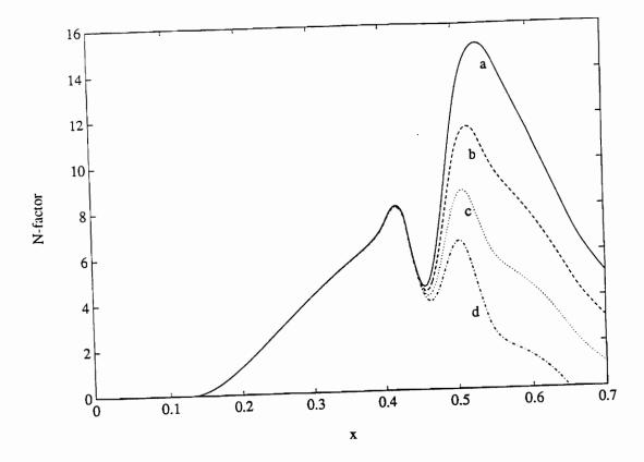
Figure 28. Influence of a suction strip on the variation of the N-factor for the most dangerous frequency with streamwise position for three suction levels when M = 0.14 a) no suction, b)  $C_q = 1.5 \times 10^{-4}$ , c)  $C_q = 3.0 \times 10^{-4}$ , and d)  $C_q = 4.5 \times 10^{-4}$ ;  $F = 35 \times 10^{-6}$ , suction strip extends from x = 0.45 to 0.53,  $h_5 = 1.0 \times 10^{-3}$ , and L3 ( $x_\ell = 0.40$  and  $x_r = 0.50$ ).
