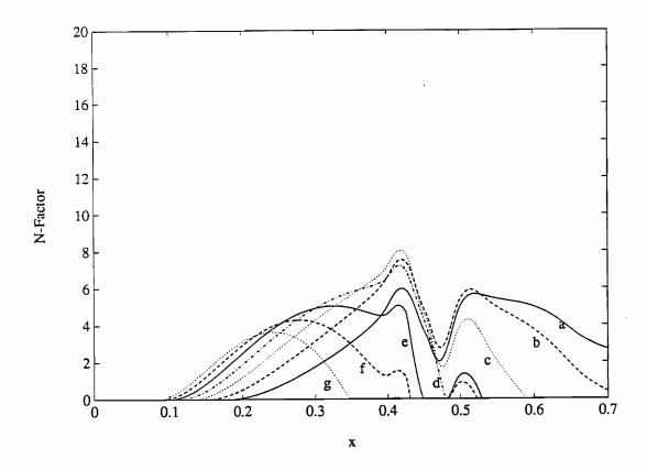
Figure 31. Variation of the N-factor with streamwise position for several frequencies with cooling for hump # 5 located at L3 when M = 0.14: a)  $F = 25 \times 10^{-6}$ , b)  $F = 30 \times 10^{-6}$ , c)  $F = 35 \times 10^{-6}$ , d)  $F = 40 \times 10^{-6}$ , e)  $F = 45 \times 10^{-6}$ , f)  $F = 50 \times 10^{-6}$ , and g)  $F = 55 \times 10^{-6}$ ;  $\Delta x_{cooling} = 0.45$  to 0.49,  $T_w/T_{ad} = 0.60$ ,  $h_5 = 1.0 \times 10^{-3}$ , and L3 ( $x_e = 0.40$  and  $x_r = 0.50$ ).
