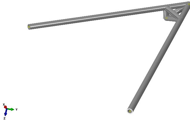
Figure 3.10: Geometry of Front Upper Control Arms (FUCA)
