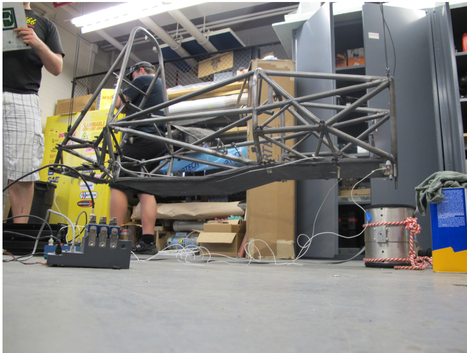
Figure 5.4: Setup of the modal test on the 2012 chassis
