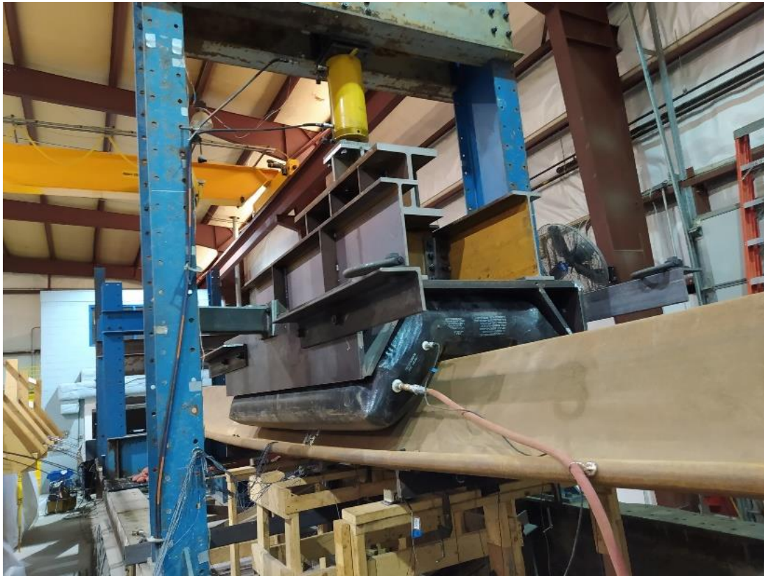
FIGURE 65: AIR BLADDER BEHAVIOR UNDER HIGH LOAD
