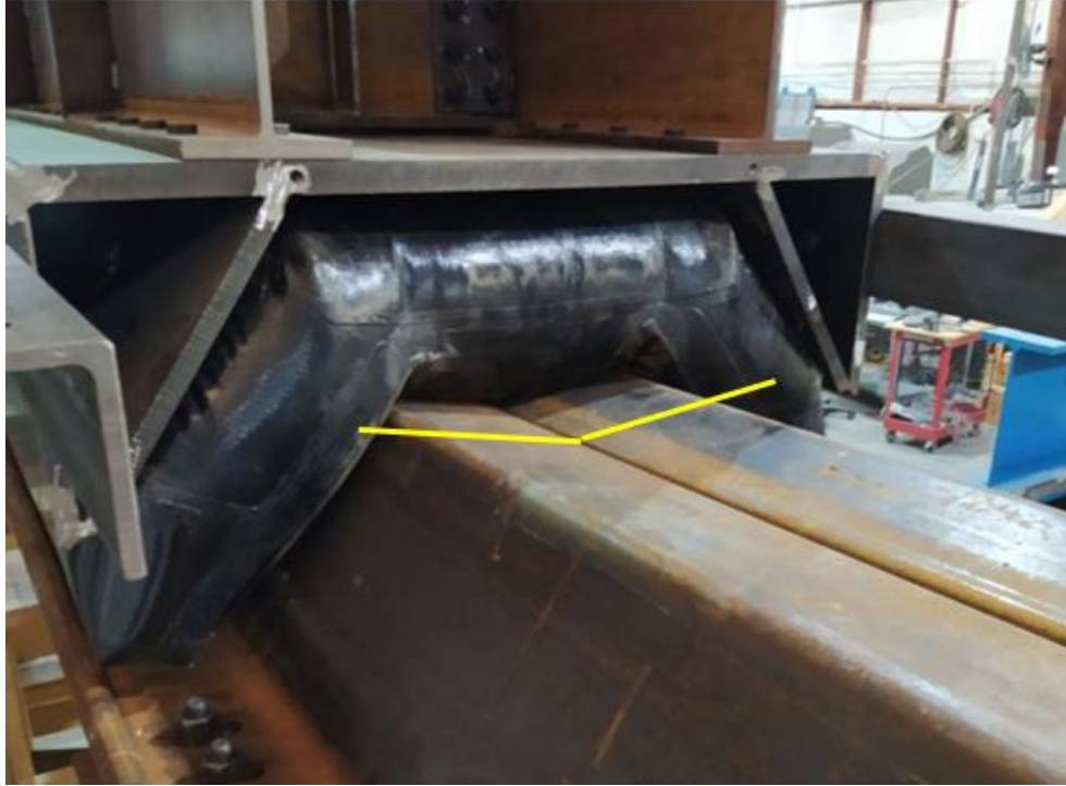
FIGURE 66: INTERLOCK BUCKLING OF XZ95-35
