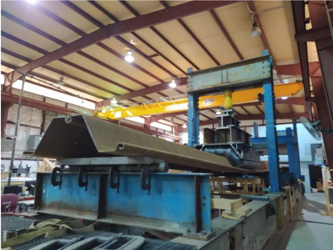
FIGURE 56: DEFORMED JZ120-35 SPECIMEN DURING TEST
