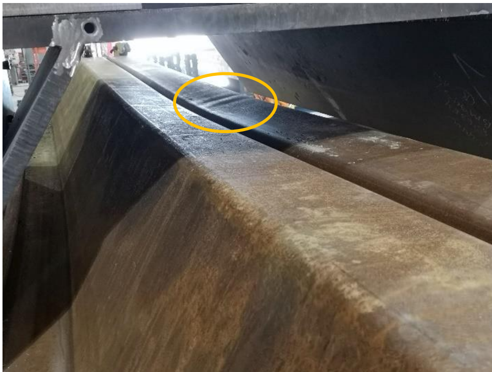
FIGURE 60: DEFORMED JZ120-16-3 SPECIMEN AFTER TEST
