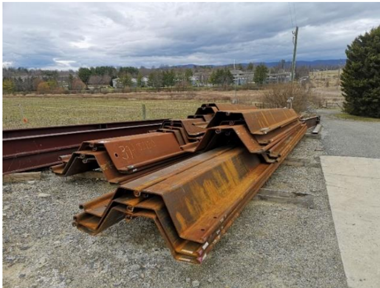
FIGURE 2: STEEL SHEET PILING SPECIMENS
