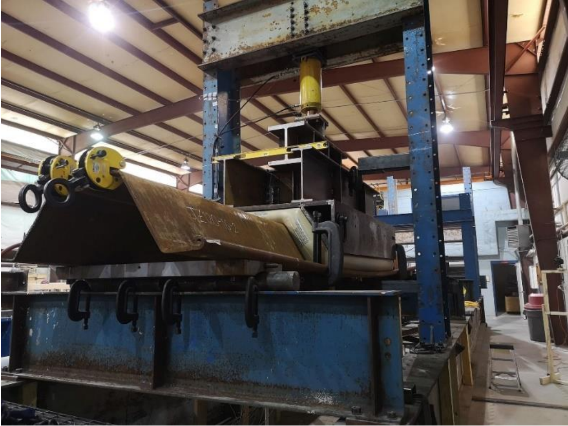
FIGURE 55: DEFORMED JZ120-16 SPECIMEN DURING TEST
