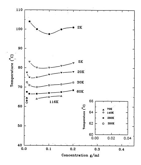
Figure 6.2.2. Cloud point temperature as a function of molecular weight for PEOX homopolymer in dilute solution. Inset is a list of cloud points of higher molecular weight PEOX polymers as listed in the literature. (ref. 4).
