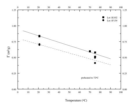
Figure 6.5.1. Elevated temperature adsorption study of PEOX  $M_{\rm w}$  = 30K homopolymer on SiO<sub>2</sub>. The cloud point of PEOX  $M_{\rm w}$  = 30K = 73 $^{\circ}$ C.
