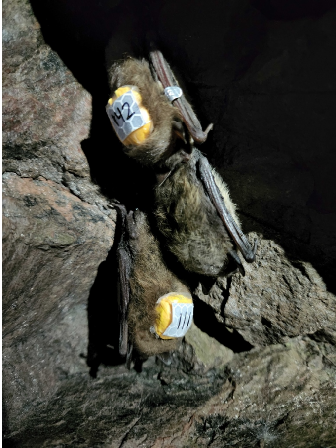
Supplemental Figure 1: Illustration of the temperature-sensitive data loggers we deployed on the backs of 287 individual hibernating little brown bats ( Myotis lucifugus ). The data loggers recorded the roosting microclimate temperature of the hibernating bats on regular intervals, capturing both torpor and arousal behavior.
