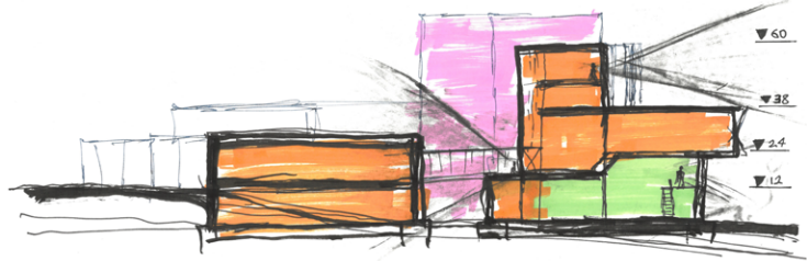
Fig. 58. Conceptual sketch exploring the stepped design and the layout of different programs around a courtyard (by author).
