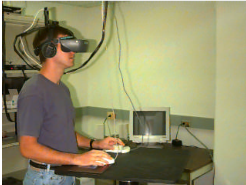
Figure 18. Experimental apparatus: VR4 worn on the head, magnetic tracking receiver mounted on top of VR4, Magellan held in the left hand, Microsoft mouse held in the right hand, and rotating platform supporting hand-held input devices.
