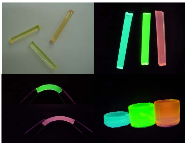
Figure 4.8. a) Transparent CdSe/ZnS-HMITFSI-PMMA composites fabricated with a 4:7 molar ratio of HMITFSI/QDs to MMA. b) Differently shaped composites exposed under an ultraviolet lamp. c) Curved composites fabricated with a 6:5 molar ratio of HMITFSI/QDs to MMA.
