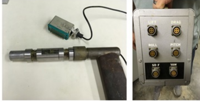
Figure 4.4: 6DOF Sting Balance SB-100 model (left), strain gauge box converter (right)
