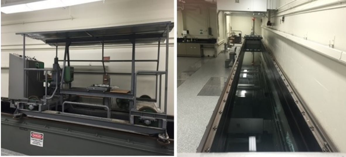
Figure 4.1: From left to right: Towing carriage and control panel unit, and towing tank
