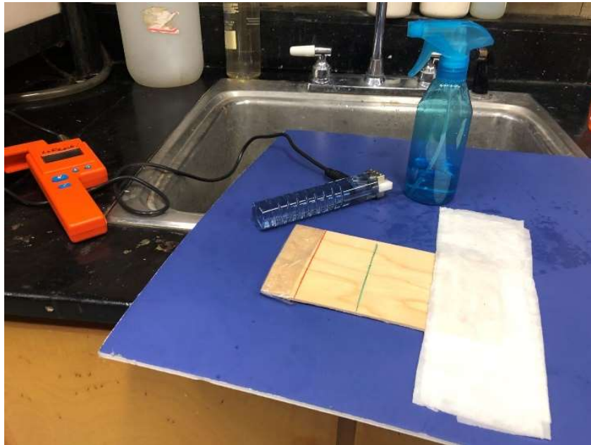
Figure 3.2.6: Experimental set up to create moisture gradients.
