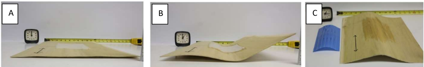
Figure 4.2.1: Photographs from qualitative monitoring of moisture-induced deformation.
