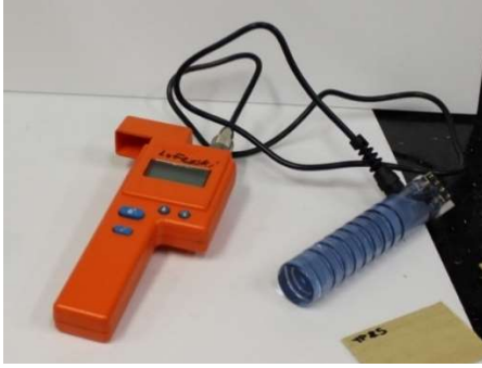
Figure 3.1.3: The Delmhorst J-2000 moisture meter and the 15-E attachment electrode.
