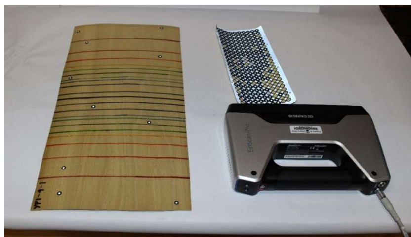
Figure 4.2.3: A sample of yellow-poplar veneer with the EinScan-Pro.
