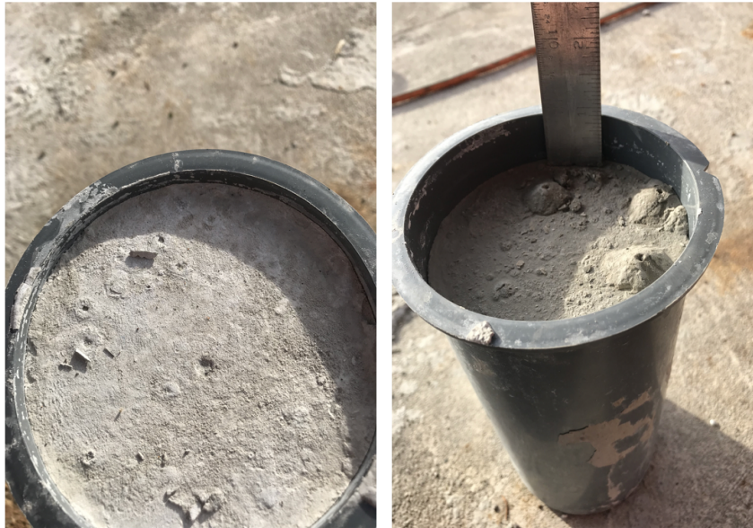
a) b) Figure 3-24 Cylinders Filled with Different Qualities of Grout
