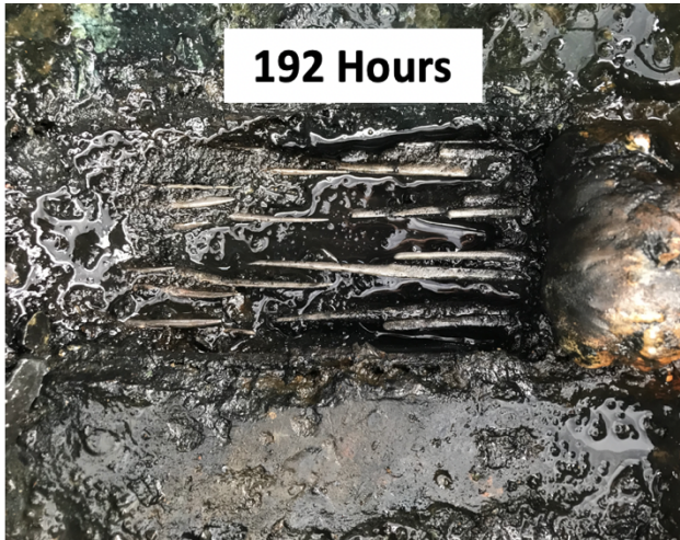
Figure 4-2 Progress in the Strand Corrosion in Poorly Grouted Duct
