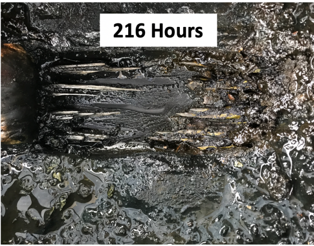
Figure 4-2 Progress in the Strand Corrosion in Poorly Grouted Duct
