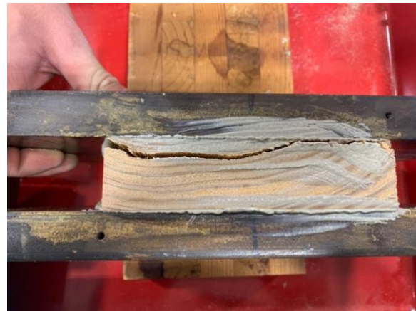
Figure 10. Rolling Shear in sample SP 7
