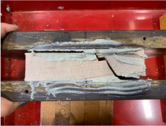
Figure 14. Rolling Shear in sample SM 2
