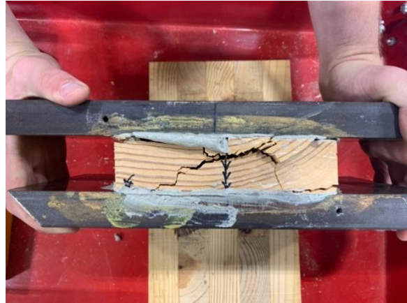
Figure 17. Rolling Shear in sample N3
