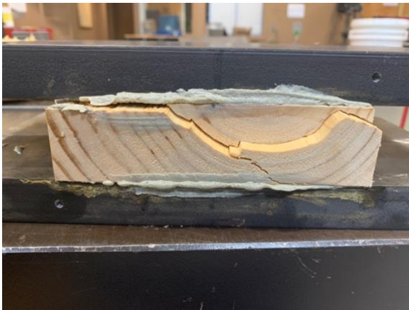
Figure 9. Rolling Shear in sample SP 2
