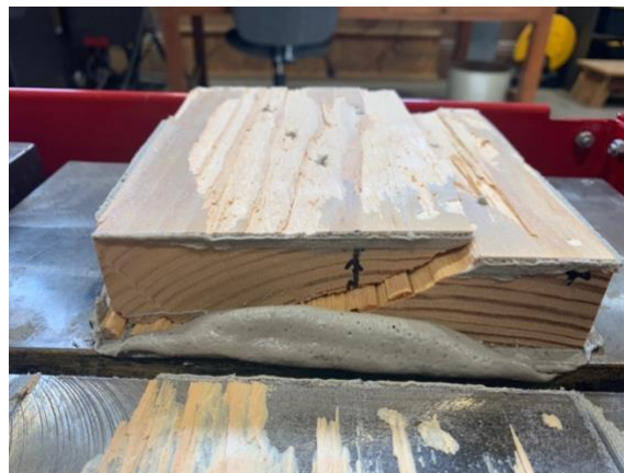
Figure 18. Rolling Shear and Adhesive Failure in sample N4
