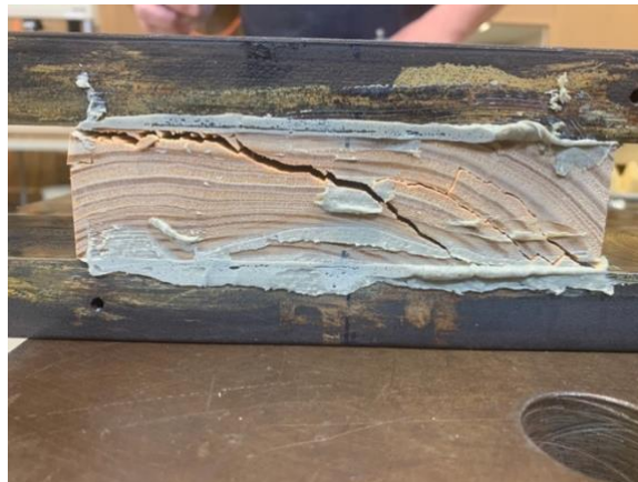
Figure 11. Rolling Shear in sample SP 11
