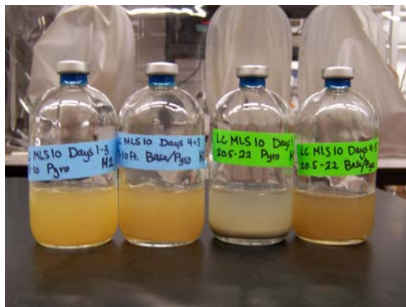
Figure 4. Photograph of the bioassays constructed for headspace hydrogen measurement using MLS10 sediment extractions. These were stored in a glovebox containing 100% ultra high purity nitrogen gas.
