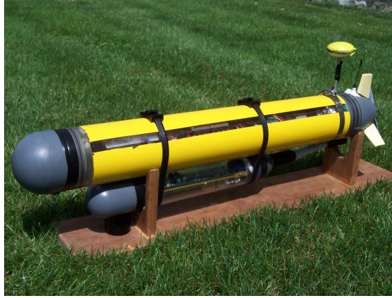
Figure 6.3: VT Miniature AUV equipped with range navigation hardware
