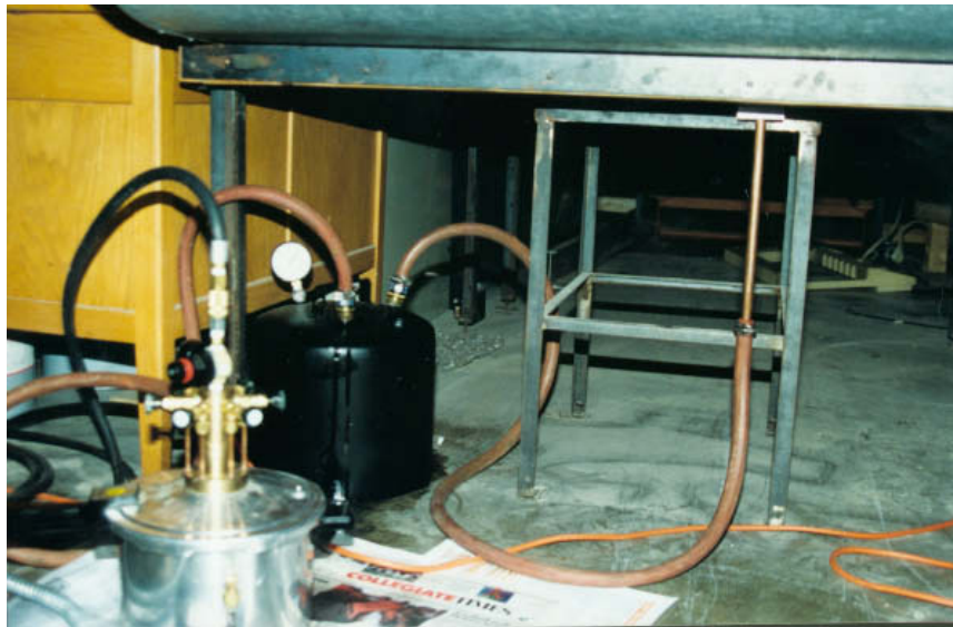
Figure 2.15: DOP generator with an impactor can under the contraction of the Cascade Wind Tunnel
