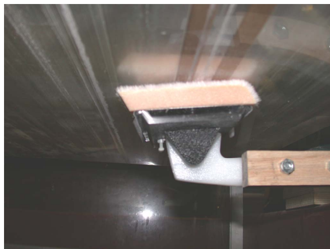
Figure 2.9: Two face to face brushes used for a moving belt
