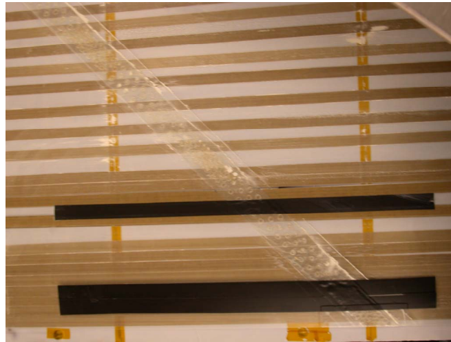
Figure 2.8: Part of the bed with high temperature tape strips for the moving belt system
