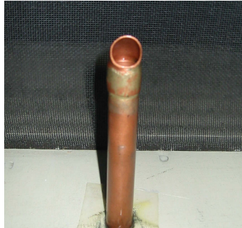
Figure 2.16: Seeding pipe downstream of flow conditioning screens in the contraction of the Cascade Wind Tunnel
