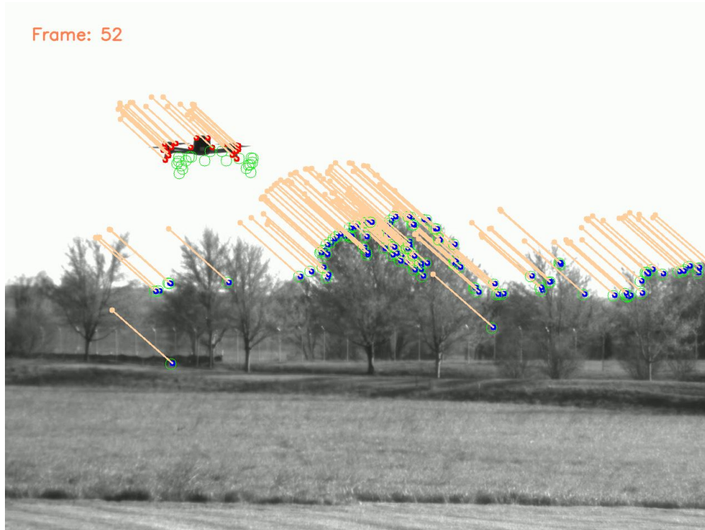
Figure 4.11: Using optical flow background estimation to identify a moving target.
