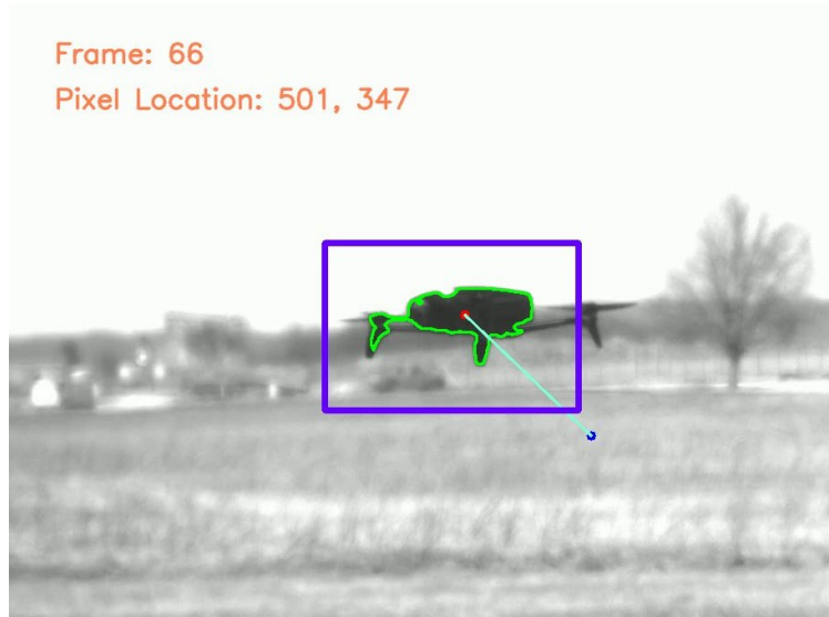
Figure 4.8: Rectangular ROI around target defining feature matching template.
