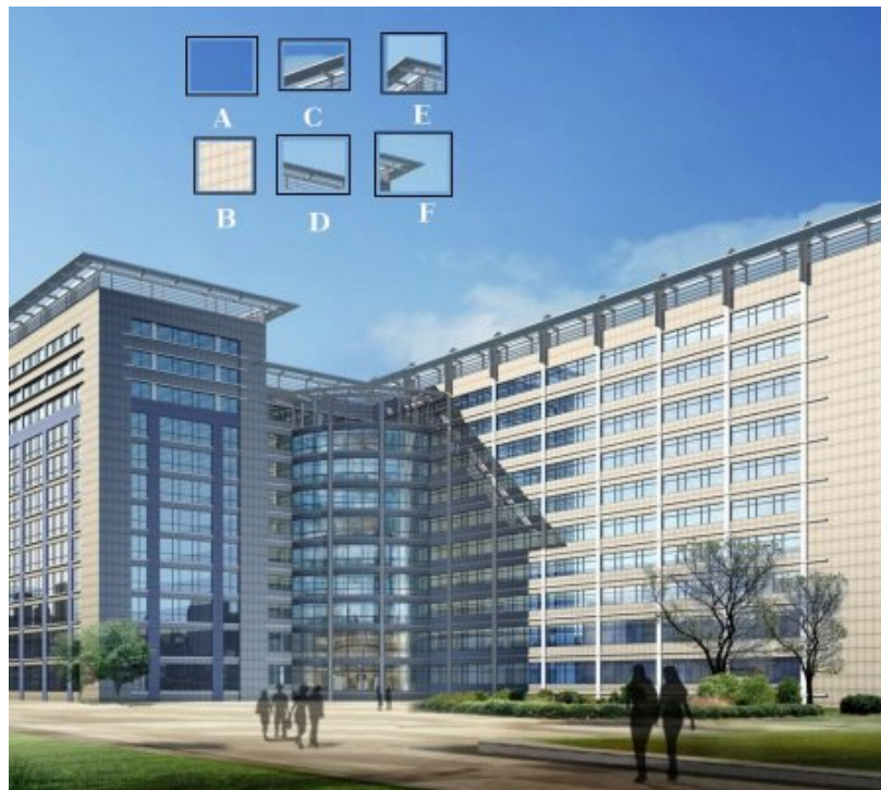
Figure 2.5: Visualization of why corners are considered good features to find and track in an image. Only templates E and F are easy to localize in the larger image. [59]
