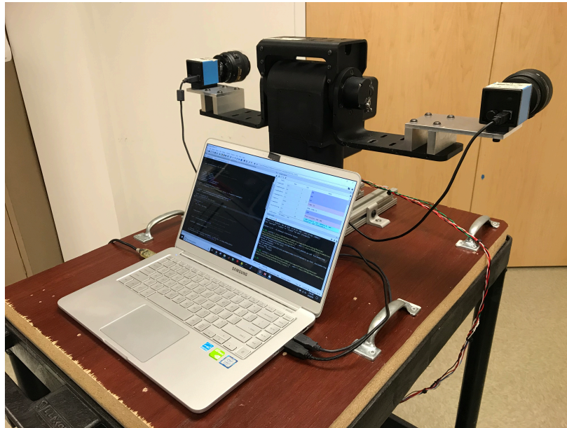
Figure 3.2: Full tracking system setup showing laptop, PTU, cameras, lenses, and cart.
