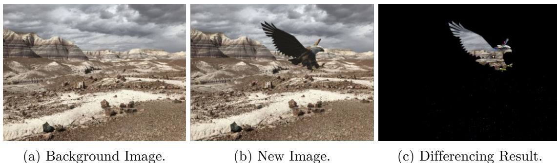
Figure 2.6: Literal differencing, in which the new image intensity array is subtracted from the background image intensity array.
