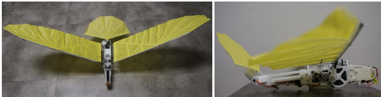
Figure 3.21: Second robotic bird prototype with lateral drive and passive wing
