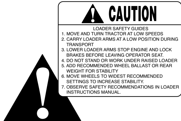
Figure 1. Typical safety sign for front-end loaders.
