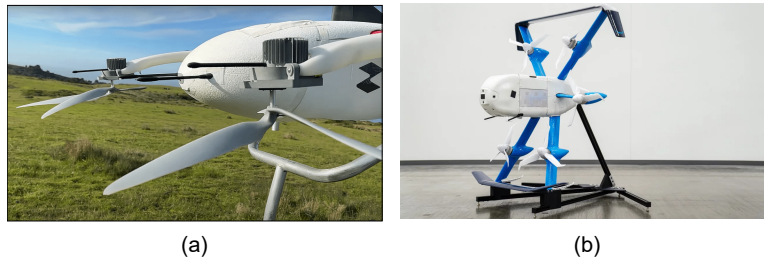
Figure 1.2: sUAS configurations: a) Zipline Platfrom 2 drone and b) MK30 drone by Prime Air
