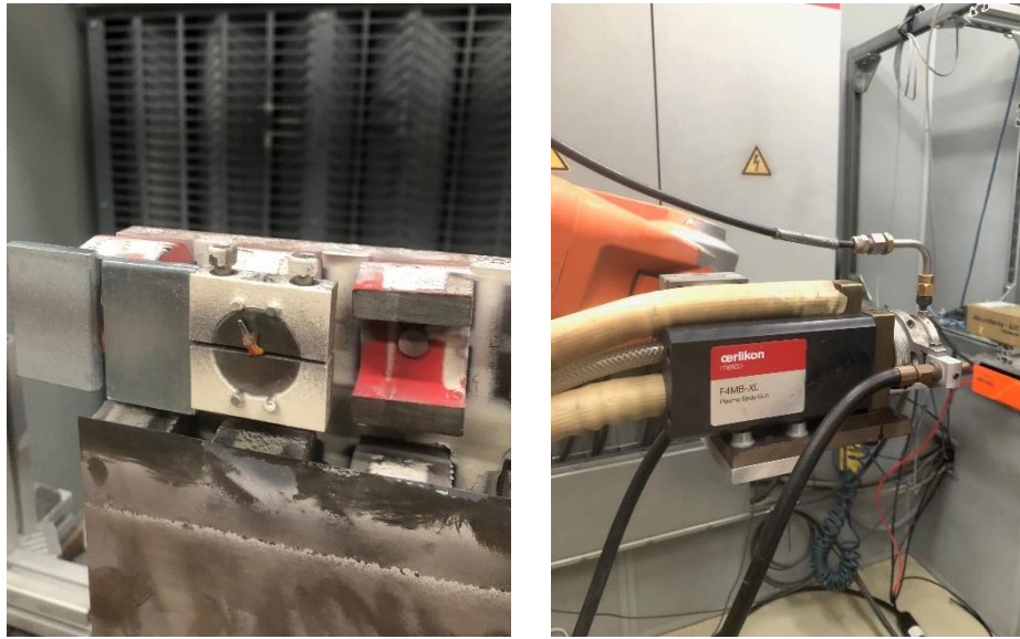
Figure 72. Photo of a) thermocouple placement within sample holder and b) the plasma spray gun used for preheating and coating samples
