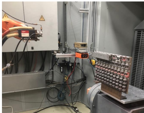
Figure 58. Plasma spraying setup used at CCAM
