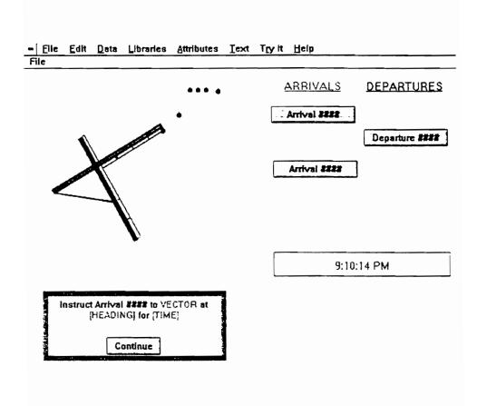
FIGURE 5.24: Screen displaying initial vectoring instructions
