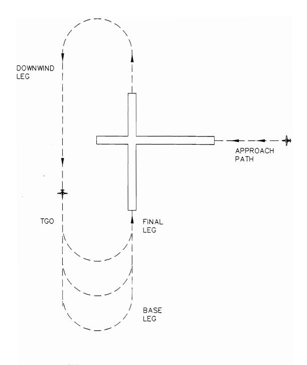
FIGURE 4.1: Diagram of Touch-and-Go Operations
