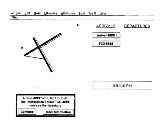
FIGURE 5.7: Touch-and-Go Advisory Screen alerting the controller of the problem
