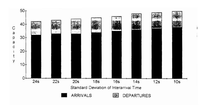
FIGURE 5.27: Saturation Capacity as it relates to Interarrival Time Standard Deviation
