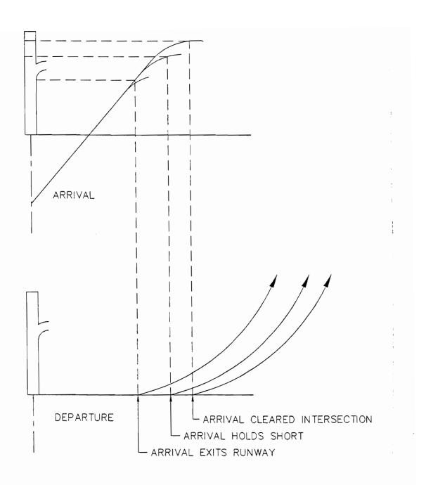
FIGURE 5.29: Time-Space Diagram for Simultaneous Intersecting Runway Operations
