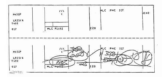
FIGURE 2.1: Depiction of a typical flight progress strip – before and after use.
