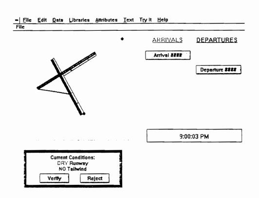
FIGURE 5.15: Display asking the controller to verify the current conditions
