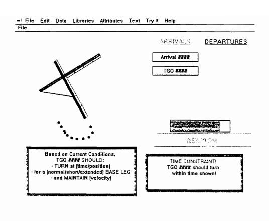
FIGURE 5.11: A disappearing bar shows time remaining to safely execute the command
