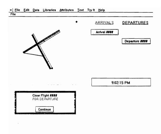
FIGURE 5.19: Display advising controller to clear flight for departure
