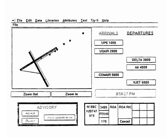
FIGURE 5.3: General Advisory Screen showing the detailed Flight Progress Strip
