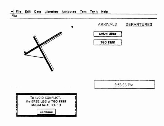
FIGURE 5.9: Advisory Screen instructing the controller to alter the TGO base leg
