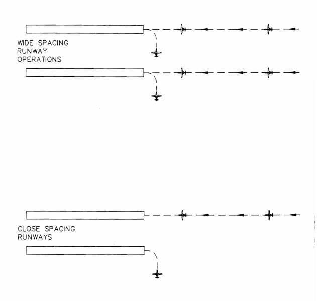
FIGURE 4.3: Diagram of Standard Bank Operations
