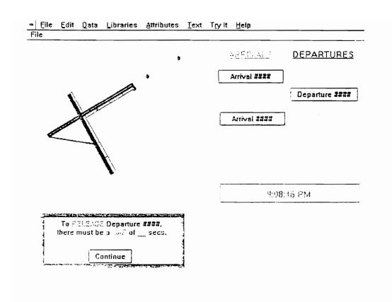
FIGURE 5.21: Advisory alerting the controller of the required gap between arrivals
