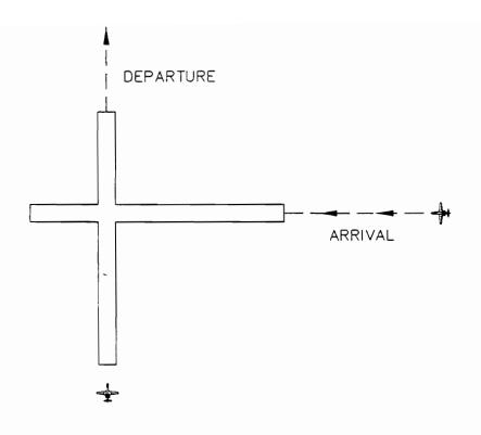
FIGURE 4.2: Diagram of Simultaneous Intersecting Runway Operations
