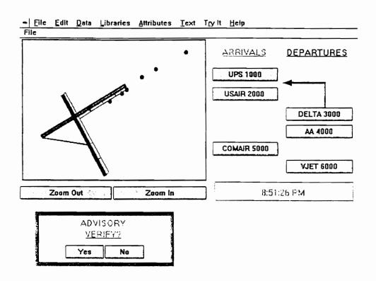
FIGURE 5.4: Screen prompting the controller for flight schedule verification
