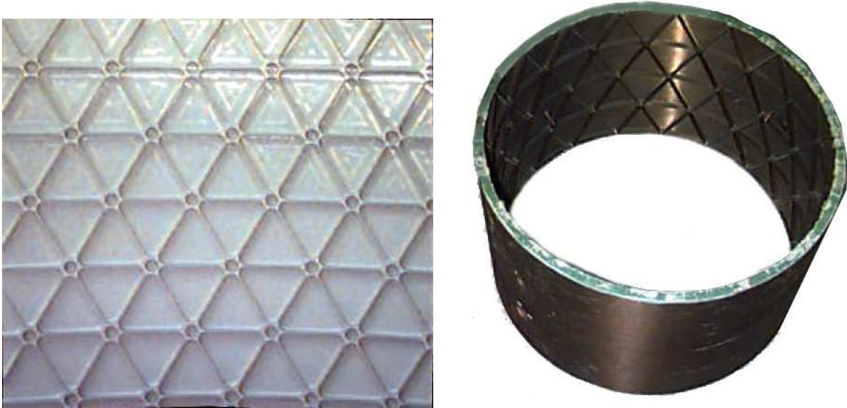
Figure 1.1: Examples of isogrid lattice structure
