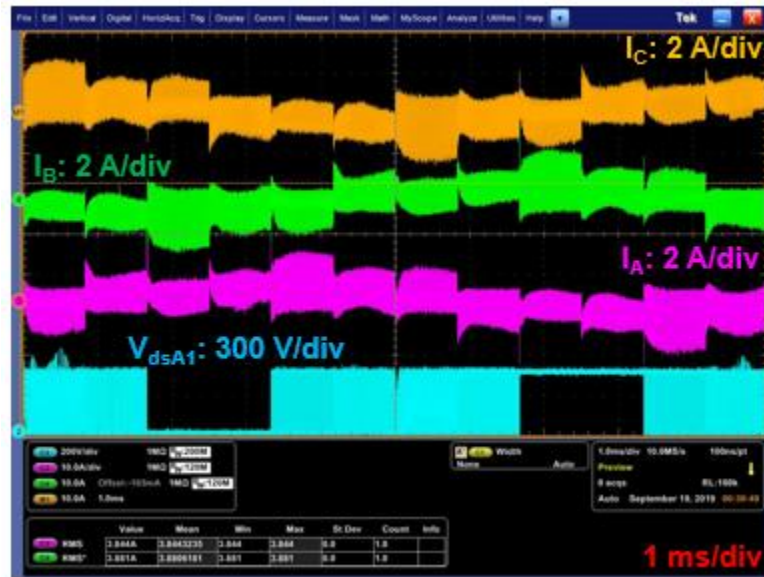
Figure 4. 40 Phase currents for V_{dc}= 300 \text{ V} , S_o=675 \text{ VA} , V_{acrms}= 86.25 \text{ V} , p.f.= 0.866 lagging
