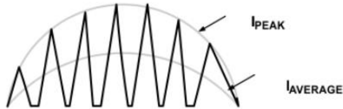
Figure 1. 14. Inductor current in DCM
