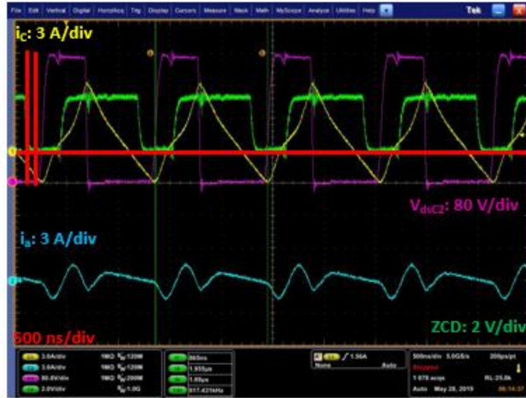
Figure 3. 54 The delays in hardware, sensing circuit and controller leading to higher negative current than desired.
