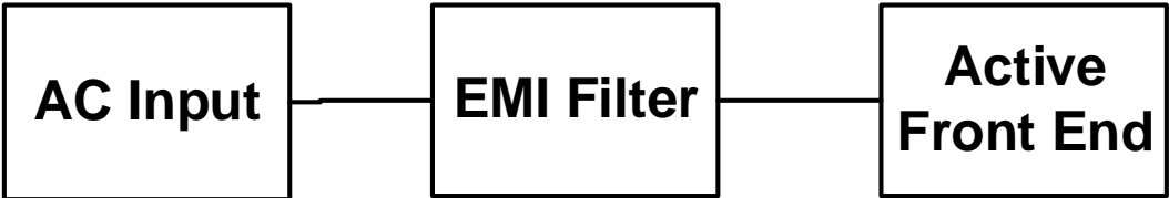
Figure 1. 2 Block Diagram of AC/DC Power Converter Systems
