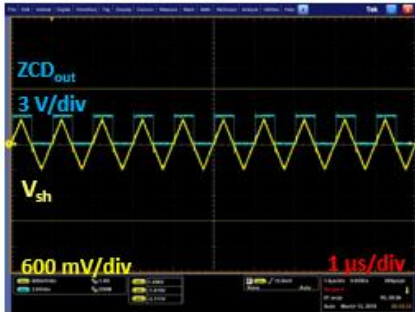
Figure 3. 52 ZCD board testing results where V_{sh} : Voltage across shunt resistor
