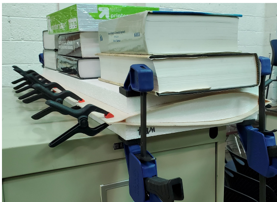
Figure 5.4: Foam core wing with balsa sheeting clamped for drying
