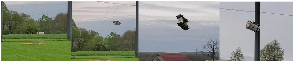
Figure 5.19: Stages of a transition flight between vertical and horizontal flight regimes [12].
