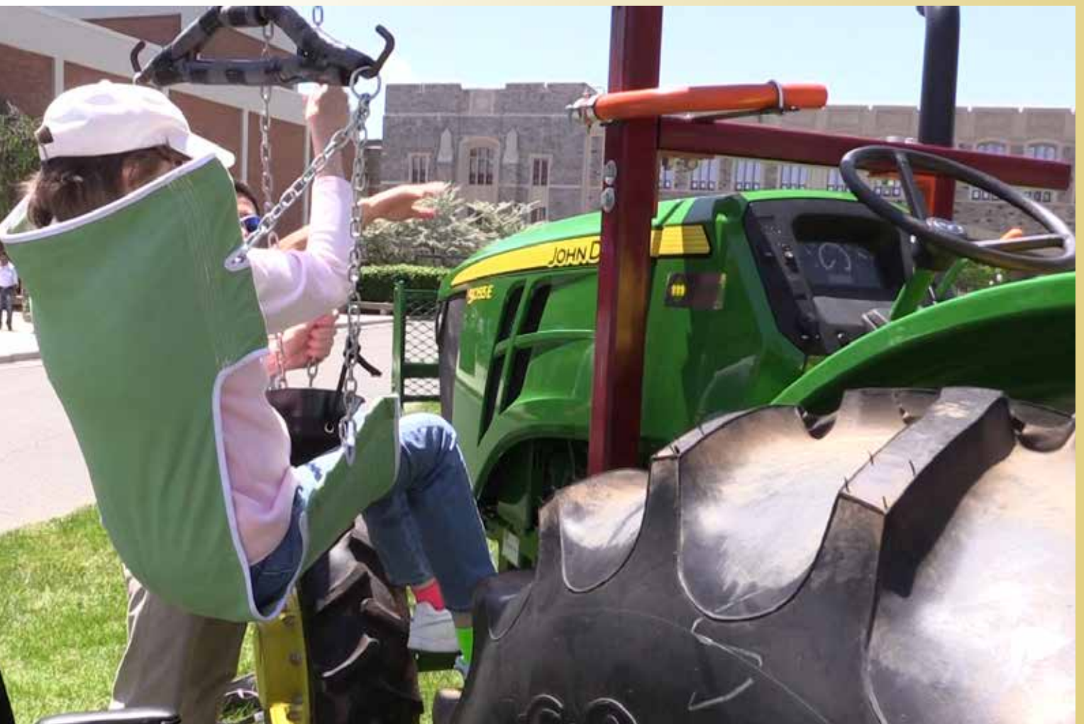
Taking on a challenge close to the roots of Virginia Tech as an agricultural college, a Senior Design team came up with an inexpensive and easy-to-use method for elderly or disabled farmers to climb into modern tractors.
