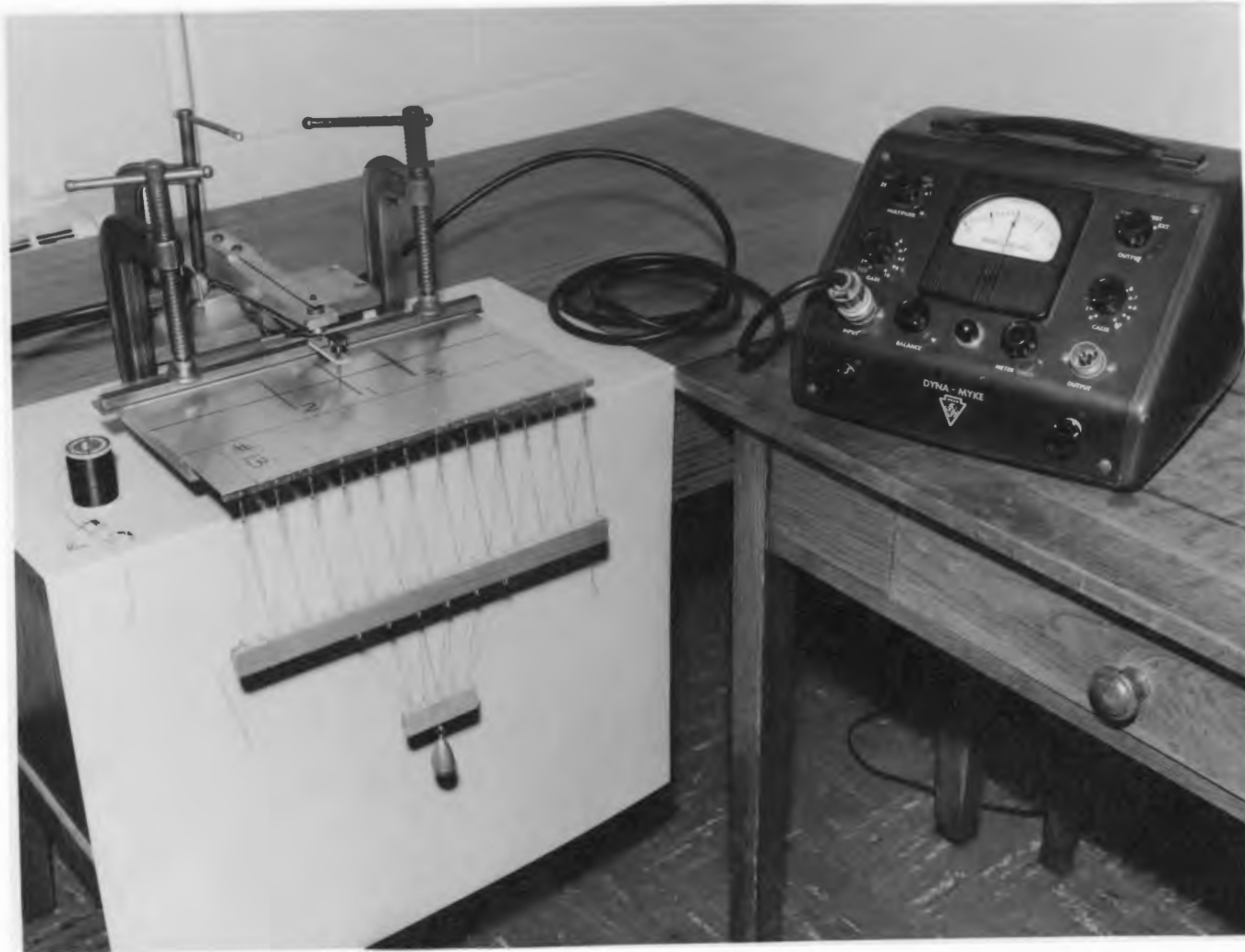
PLATE 9.1 TEST SETUP WITH LOADING FIXTURE, LVDT, AND FIXED EDGE
