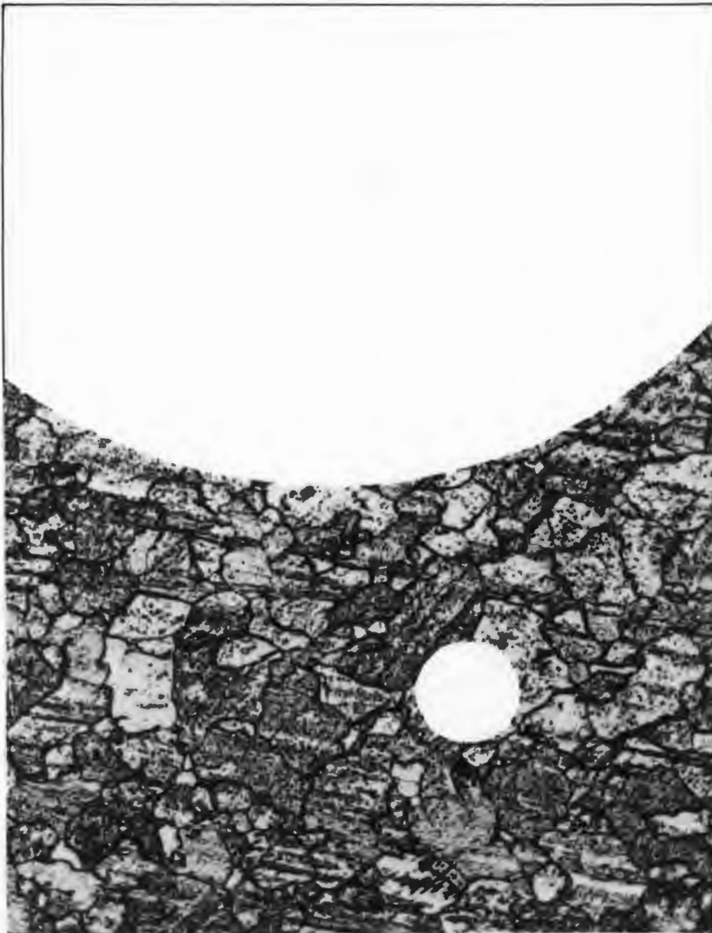
PLATE 11.1 STEEL STRUCTURE WITH LARGE (.02") AND SMALL (.002") HOLES
