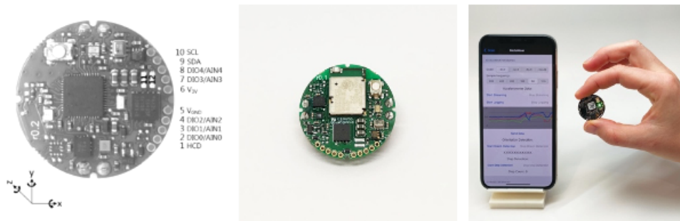
Figure 3.1: The MMC circuit board (left and center), a hand holding a coin next to a cell phone (right). The pictures are courtesy of MBIENTAB ( https://mbientlab.com ).
