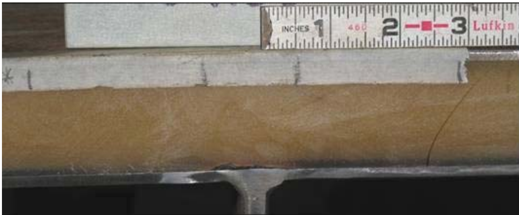
Figure 5.6 Panel B failure, elastomer core crack
