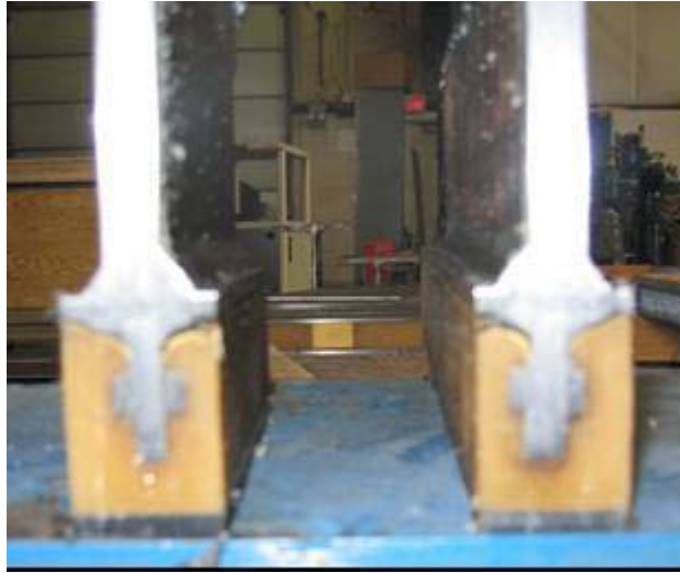
Figure 4.5 Shear studs in Panel 4
