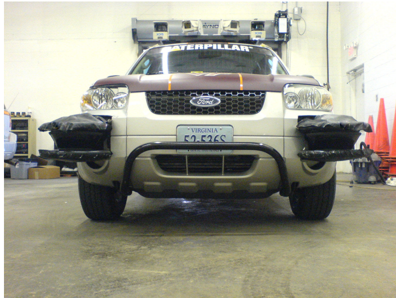
Figure 2.2: The protection for the Ibeo XT's is designed to break away from the vehicle in the event of a collision.
