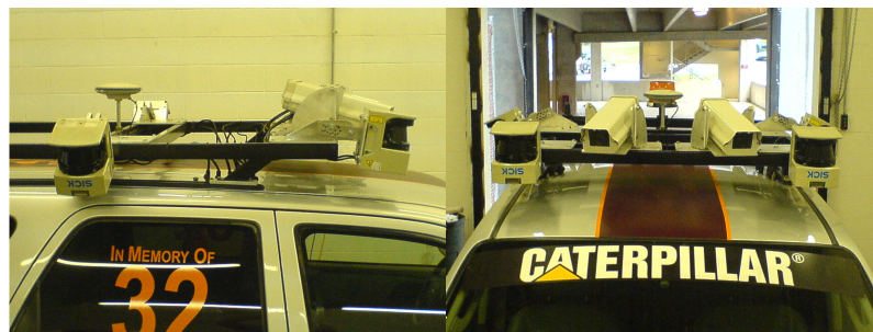
Figure 2.3: The sensor mounts on the roof rack are designed such that the orientation of any one sensor can be easily adjusted.
