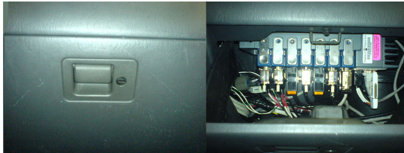
Figure 2.1: The RIO has been installed in the glove compartment space to preserve the aesthetics of the vehicle interior.
