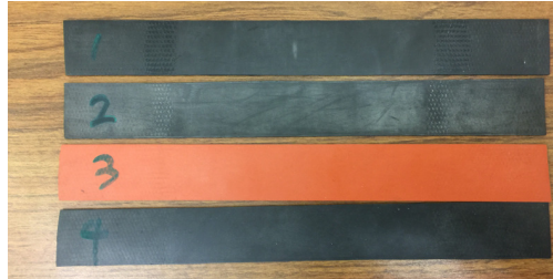
Figure 5.10: Polymer Samples 1-4 for Tests. Sample 1: Multipurpose Neoprene Rubber, 70A. Sample 2: Multipurpose Neoprene Rubber, 60A. Sample 3: High Temperature Silicone Rubber. Sample 4: Oil Resistant Rubber, 50A.
