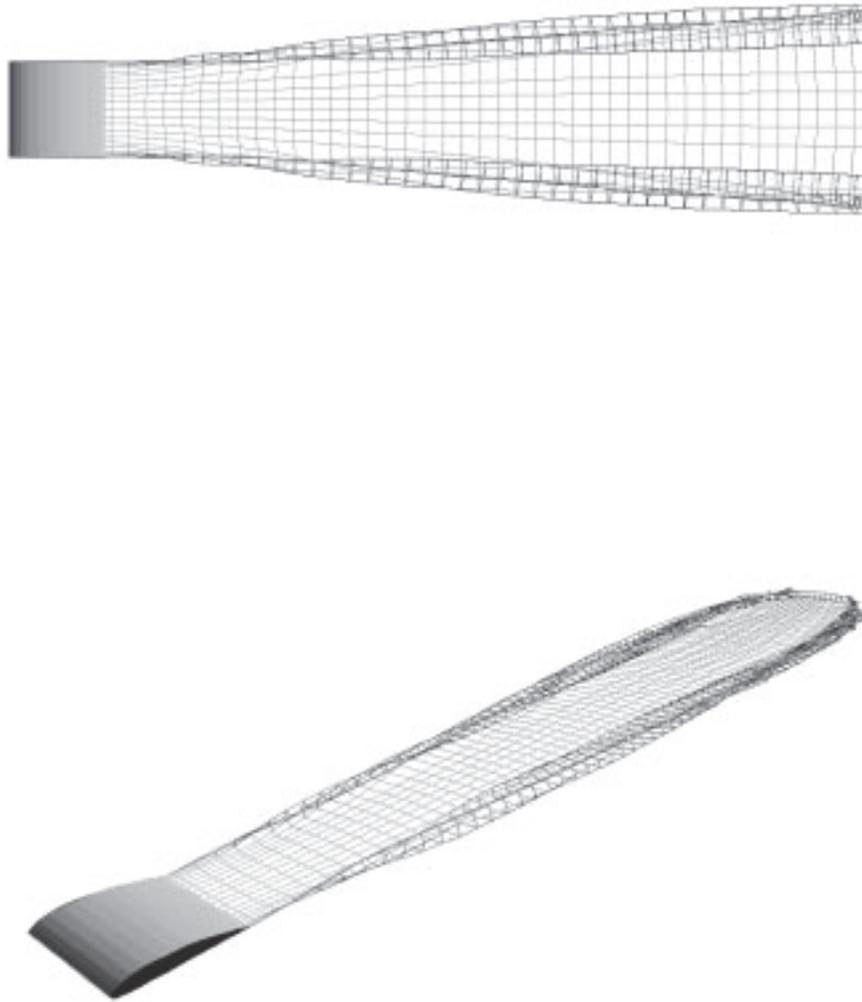
Figure 2.40: Flow Over A ClarkY Airfoil (AR=1.0) In Ground Effect; Doublet Panel Method
