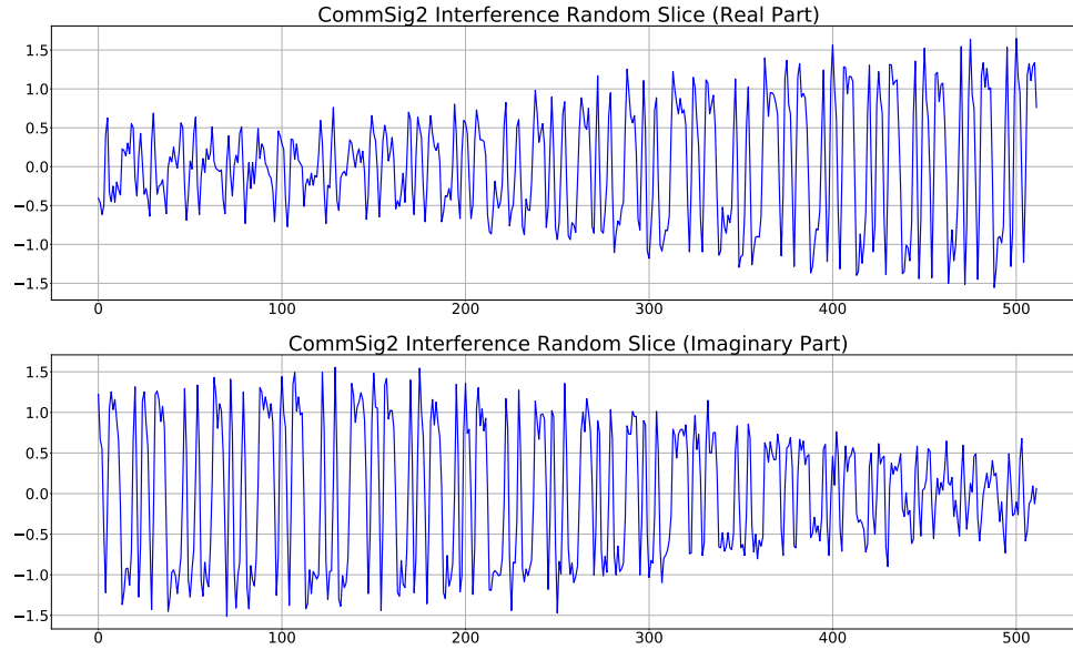
Figure 5.3: Real and Imaginary Plots of CommSignal2 Digital Communication Signal
