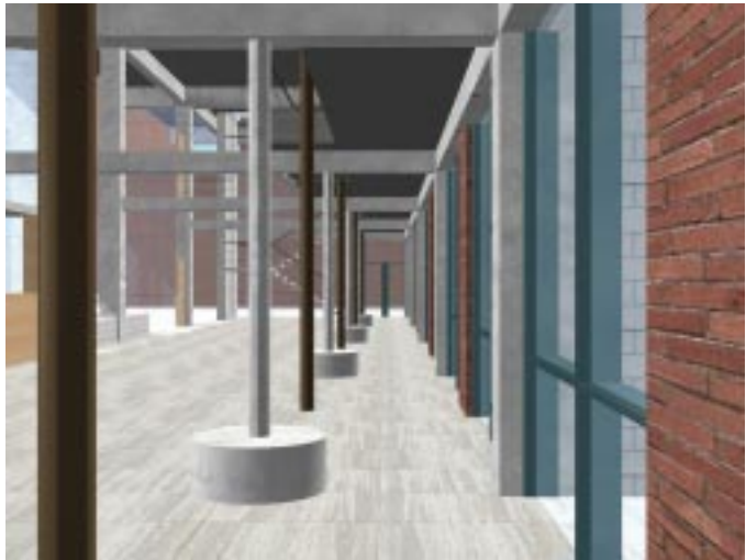
alternating steel and concrete columns and shop glass wall
