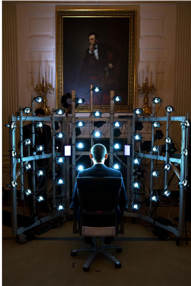
Figure 1.5: Array of lights and cameras used to capture the 3D information of President Obama's face. That information was then used to create the bust in Figure 1.4 (taken by Pete Souza).[\[14\]](#)
