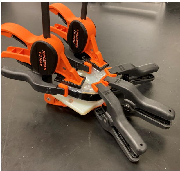
Fig. 2 Spring clamps provided “bite” force for fitting the boil-and-bite mouthguard to the 3D-printed dentition
