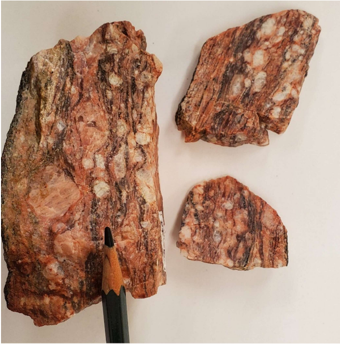
Figure 2.5. Polished slabs of sheared leucogranite sample RM-22-3. Note rigid pink feldspar porphyroclasts around which ribbons of plastically deformed quartz and trails of comminuted feldspar fragments anastomose. Slabs cut perpendicular to mylonitic foliation and parallel to geographic horizontal.
