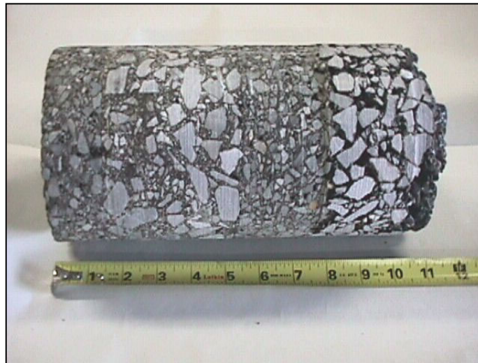
Figure 5-1: Typical HMA Core Extracted from Section H at the Virginia Smart Road
