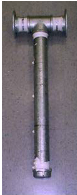
Figure 4.32. Picture of quarter-wavelength tube used during this study
