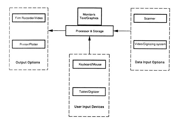
Figure 6.2. A proposed model of the hardware platform for a computer aided Inventory and Facility Management system
