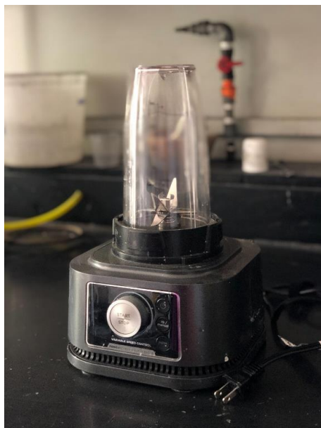
Figure 5.2 The Ninja blender used for the blunging process.
