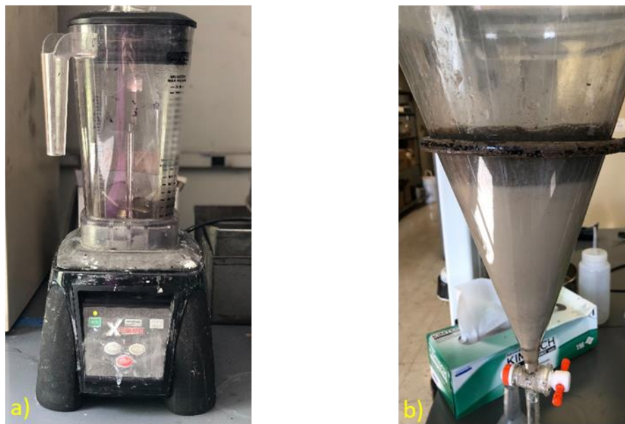
Figure 5.3 a) The high-shear Waring blender for the HHS process; b) phase separation in the separatory funnel after one HHS test.
