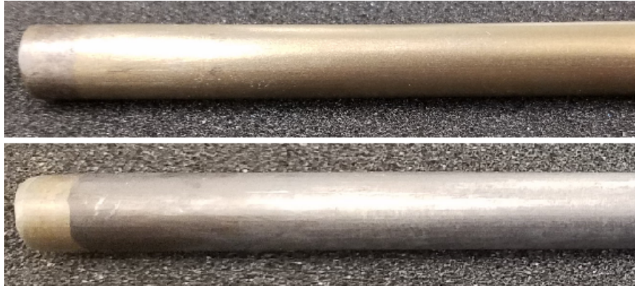
Figure 5.4: Monel rodlet before (top) and after (bottom) multiple quenchings
