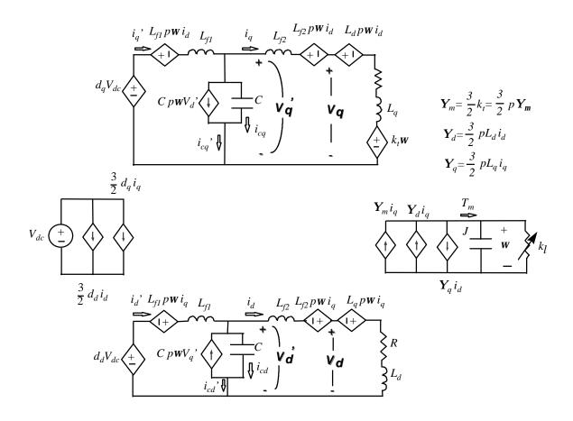
Figure 18. VSI fed PMSM drive (plant) d-q average model with a VSI output filter
