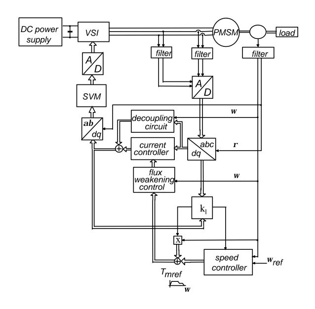
Figure 22. Reference motor torque and speed controller adjustments to active load for the speed loop stabilization
