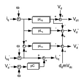
Figure 20. Decoupling scheme for the PMSM drive with a VSI output filter
