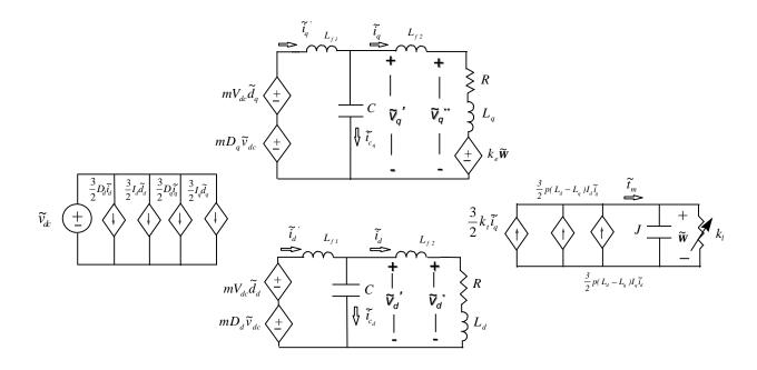
Figure 21. Dq small-signal average model of the linearized VSI-fed PMSM system with a three-phase EMI filter and without back emf elimination
