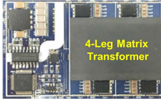
Fig. 3.6. Hardware prototype of 400V/12V LLC with proposed shielding.
