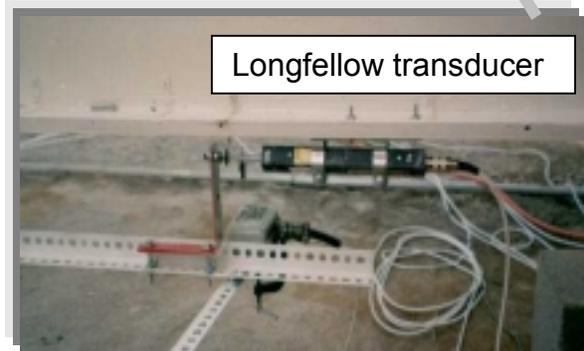
Figure 3.7. Instrumentation in place for measuring deflections during lateral load test.
