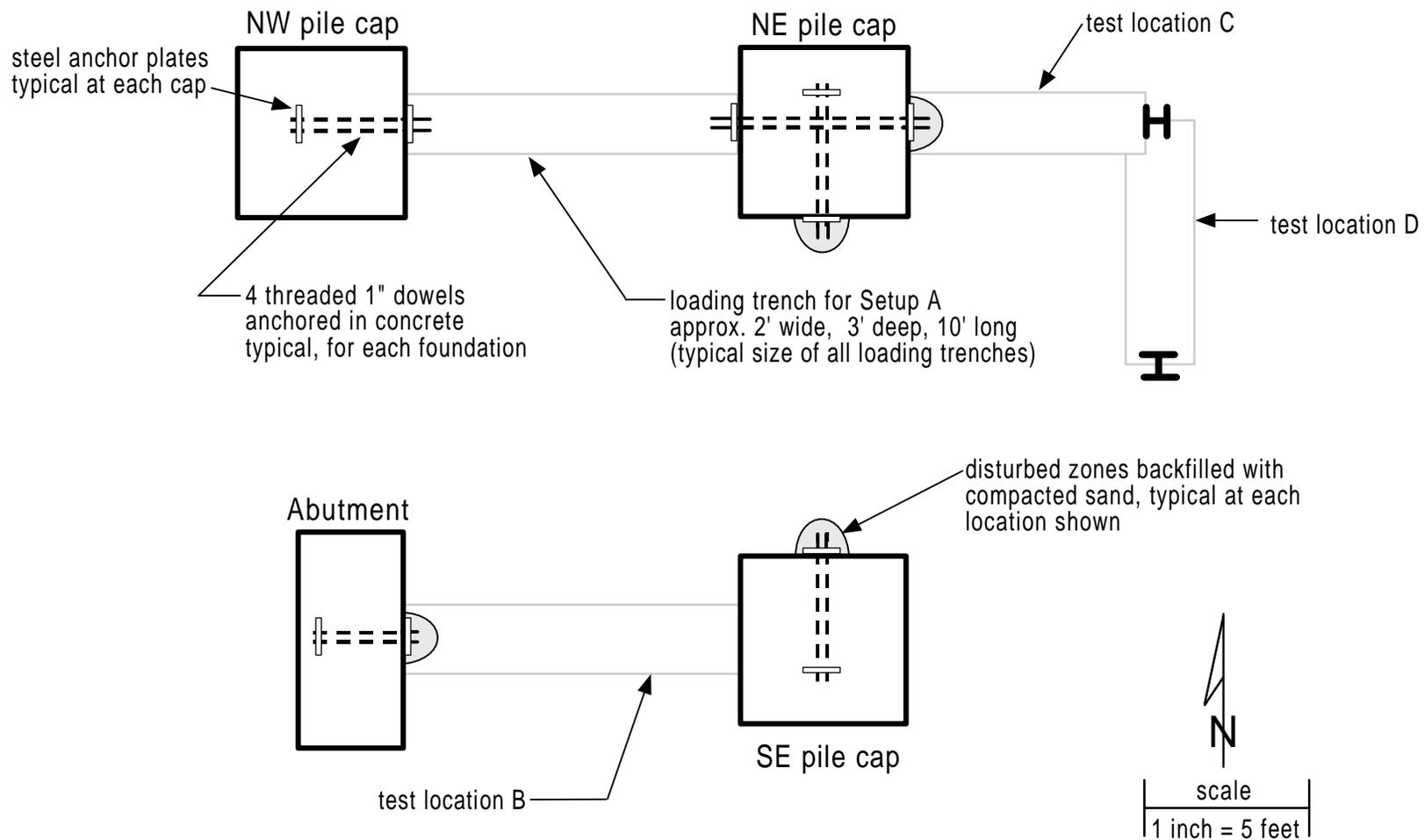
Figure 3.3. Plan view of anchor rod layout.
