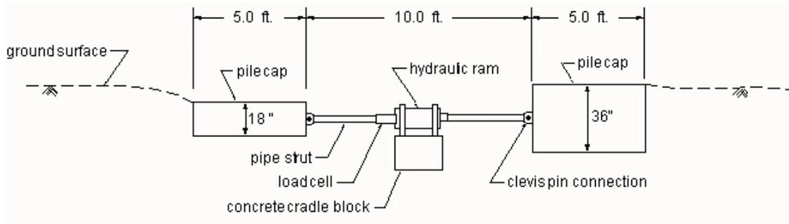
Figure 3.5. Hydraulic ram and steel struts positioned in loading trench.
