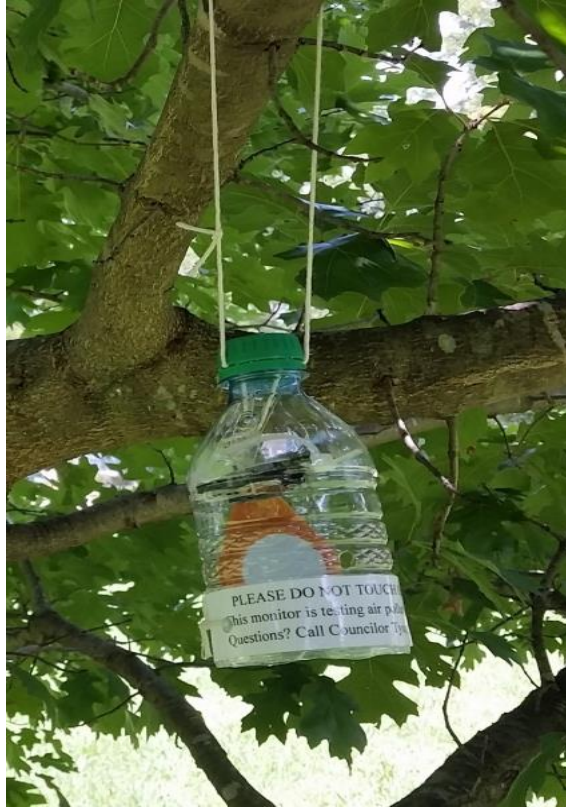
Figure 2.9.1. Picture of deployed passive organic vapor monitor and iButton with plastic housing.
