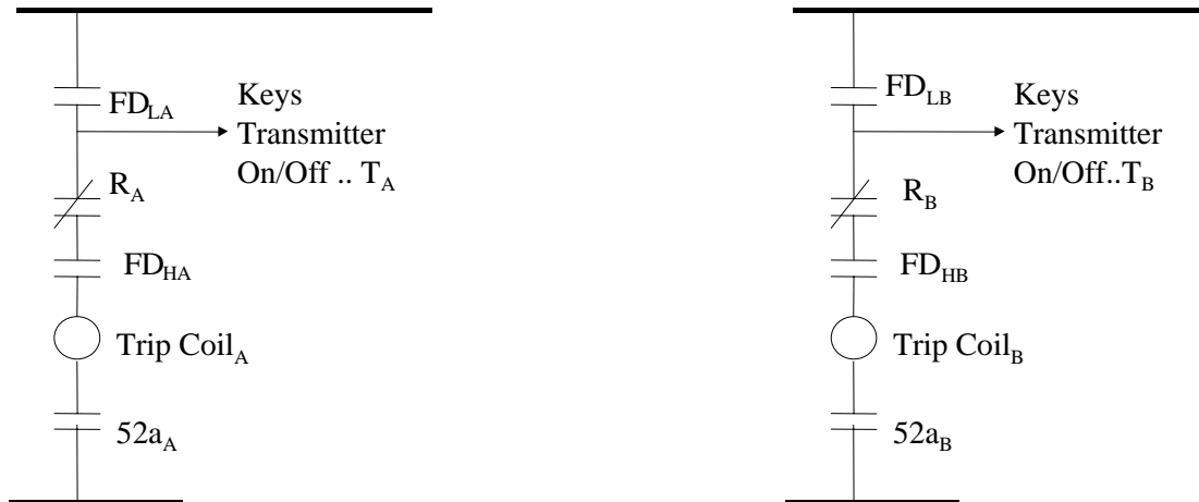
Figure 28: DPCB logic schematic, for A and B line sides.
